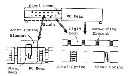
Fig.3 Rigid Body-Spring Element Model
