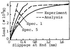
Fig. 5 Load vs. Slippage at End
