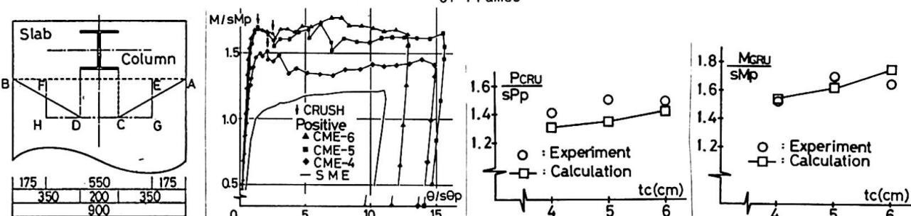
Fig. 6 Effective Width of Concrete Slab      Fig. 7 Moment - Rotation of Beams      Fig. 8 Story Shear Force upon Concrete Crushing      Fig. 9 Moment upon Concrete Crushing
