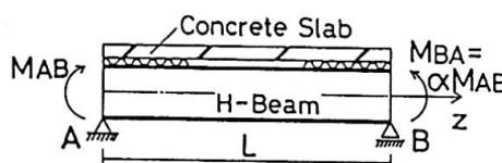
Fig. 5 Composite Beam for Analysis
