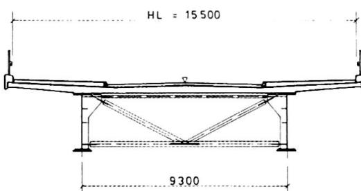
*Jyväsjärvi bridge. Cross-section of deck structure. Due to lateral preressing it has been possible to use only two main beams.*
