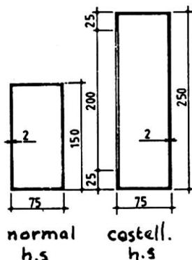
A comparison between two beams with the same use of material gives the following ratios between some characteristic values.
