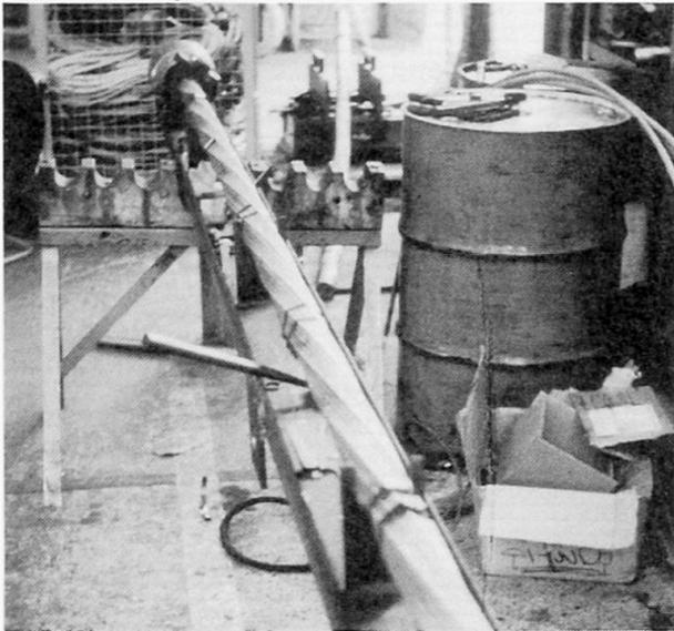
Fig. 2 Twisted Test Bundle with Long Lay Length
