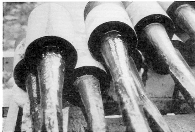
Fig. 5 Finished Sockets after Casting
