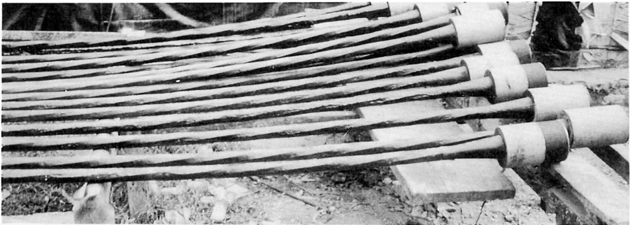
**Fig. 1** Novel Parallel Wire Bundles with Long Lay Length Twist, Polyurethane Coating and Zinc Alloy Cast Socket
