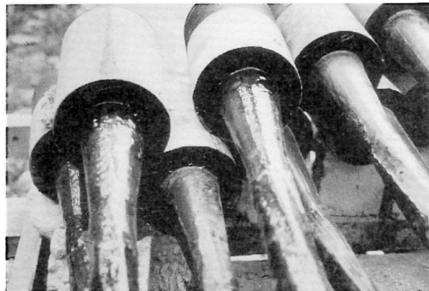
Fig. 5 Finished Sockets after Casting
