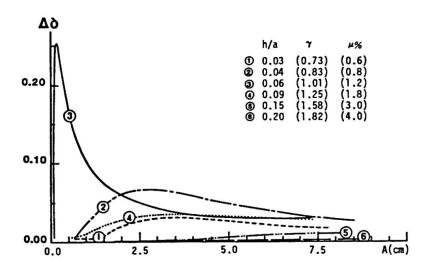
Fig. 3 Additional damping due to TLD
