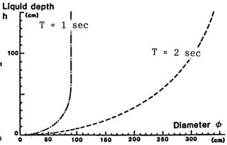
Fig. 9 Required depth versus container diameter
