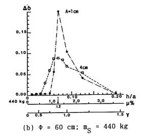
$\underline{\text{Fig. 4}}$  Comparison of TLD for the diameters 40 cm and 60 cm
