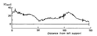
Fig. 6 -  $C_{\rm ovt}$  coeff. on a wheelset for the train entering the bridge
