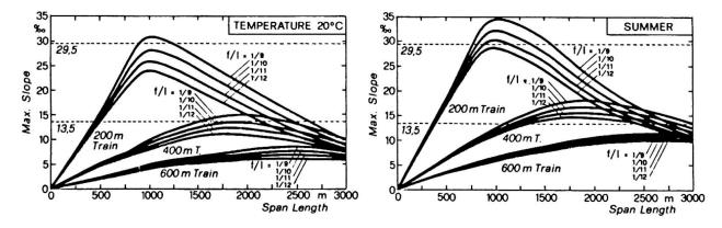
Fig. 3 - Maximum slopes versus centre span length, reference temperature
