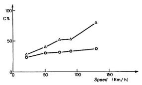
Fig. 10 - C  $_{\rm ovt}$  (O) and C  $_{\rm d}$  ( $\Delta$ ) maximum values versus train speed
