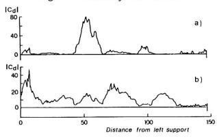
Fig. 7 -  $C_d$ , train entering the bridge: a) right wheel b) left wheel
