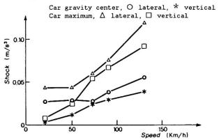
Fig. 9 - Maximum carbody shock
