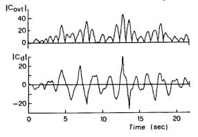
Fig. 12 -  $C_{\rm ovt}$ ,  $C_{\rm d}$  for train running on the bridge during a seismic event
