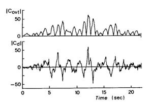
Fig. 11 -  $C_{\rm ovt}$ ,  $C_{\rm d}$  for train running on ground during a seismic event
