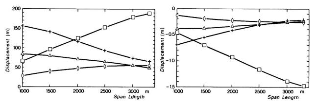
Fig. 1 - Maximum vertical displacements versus centre span length
