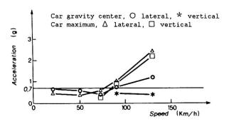
Fig. 8 - Max. lateral carbody accel.
