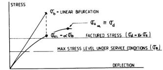
Fig 3.1 Definition of safety requirements
