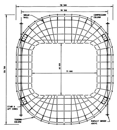
Fig. 1 Layout of Fixed Grandstand Roof
