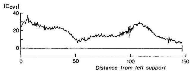
Fig. 6 -  $C_{overt}$  coeff. on a wheelset for the train entering the bridge
