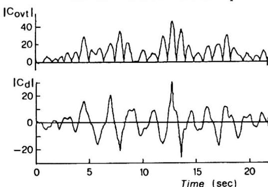
Fig. 12 -  $C_{overt}$ ,  $C_d$  for train running on the bridge during a seismic event
