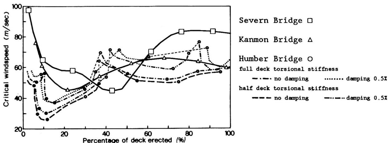
Fig. 5 - Critical windspeed versus percentage of deck erected
