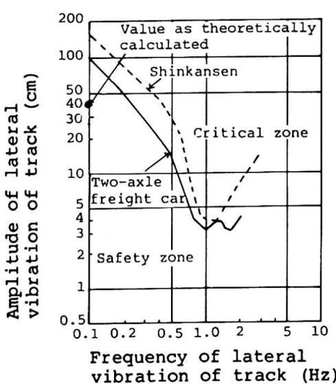
Fig. 4 Running Safety Limit Curve
