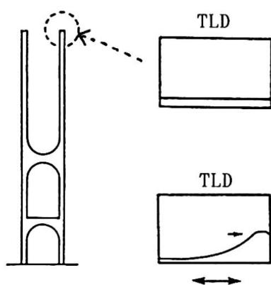
Fig. 1 TLD installed on a bridge tower
