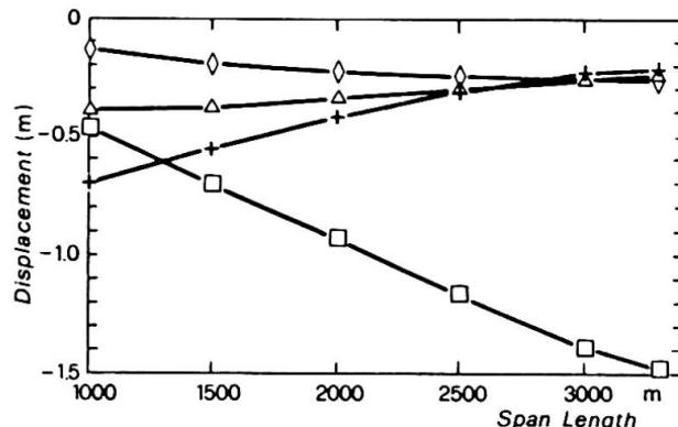
Fig. 2 - Minimum vertical displacements versus centre span length
