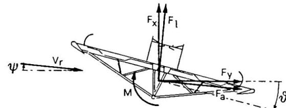
Fig. 7 - Aerodynamic forces
