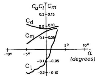
Fig. 10 - Aerodynamic coeff. with closed grid
