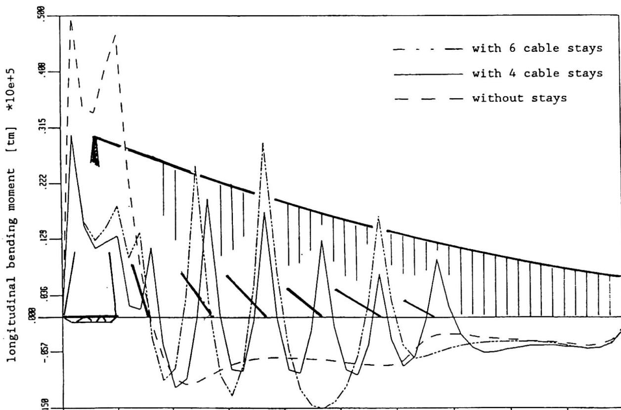
Fig. 4: deck bending moment for different configurations
