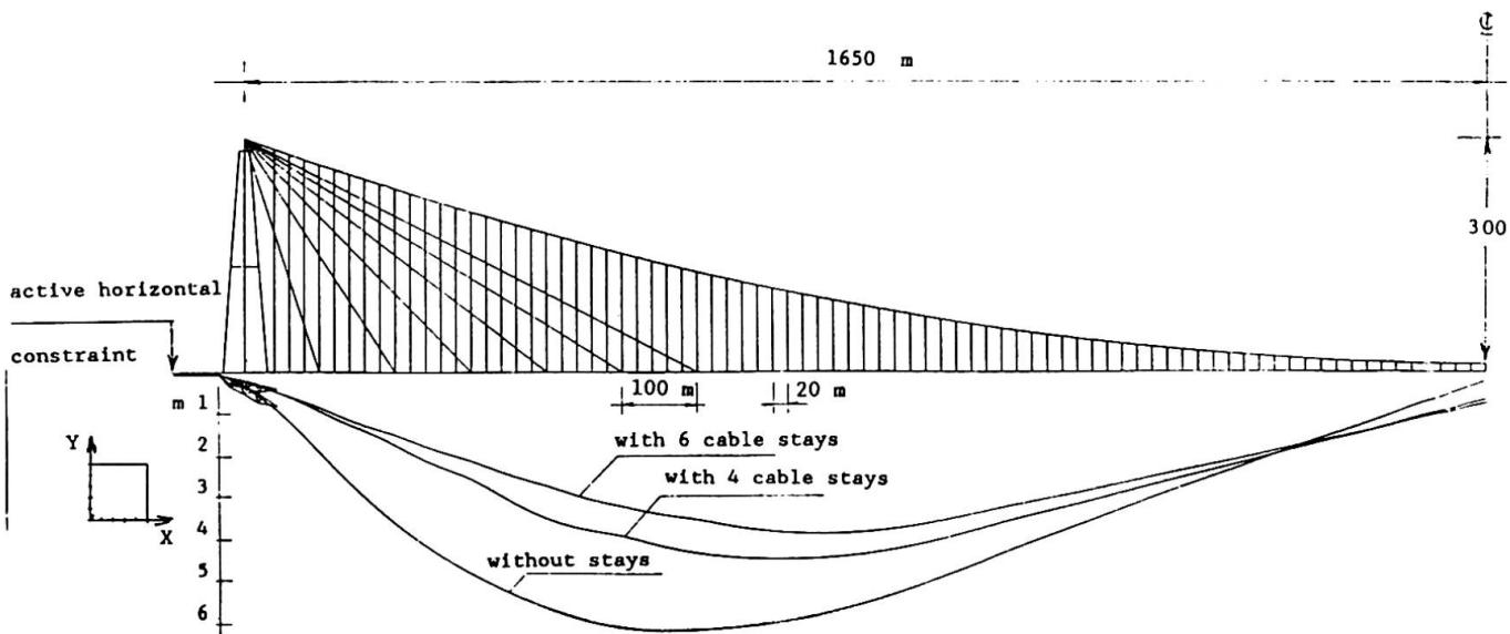
Fig. 3: deck deformed shape for different shapes
