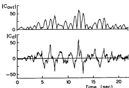
Fig. 11 -  $C_{overt}$ ,  $C_d$  for train running on ground during a seismic event
