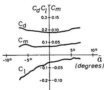
Fig. 9 - Aerodynamic coeff. with open grids
