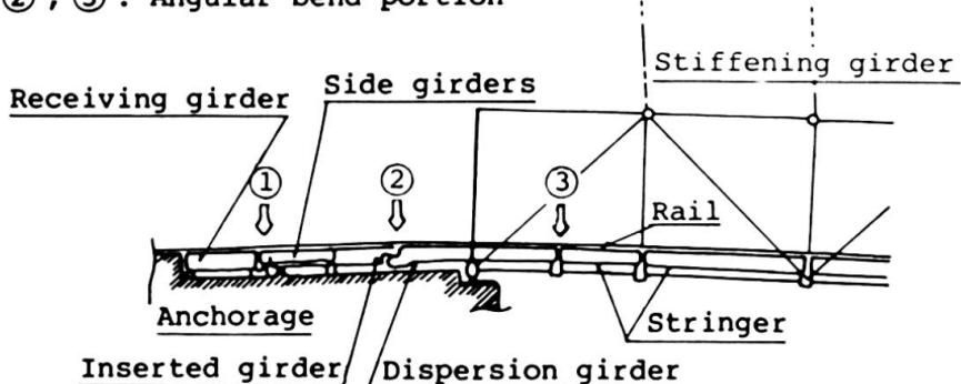
Fig. 3 Transit Girder System of Inserted Girder Type
