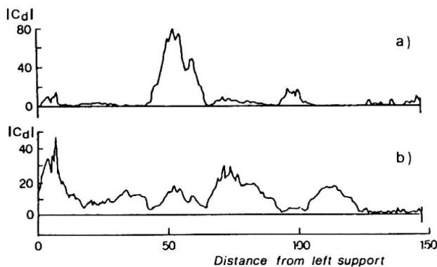
Fig. 7 -  $C_d$ , train entering the bridge: a) right wheel b) left wheel
