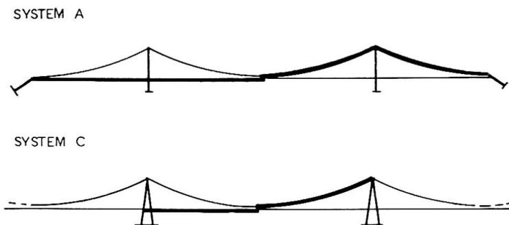
Fig. 3: Stabilization of the cables at midspan by longitudinal fixation.
