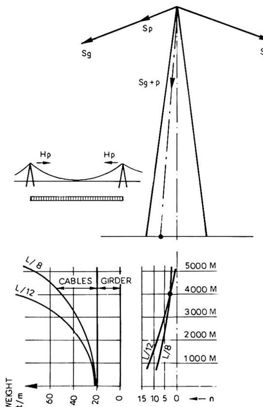
**Fig. 2:** Resultant forces in pylons for suspension system C and road traffic for cable sag L/8 and L/12.
