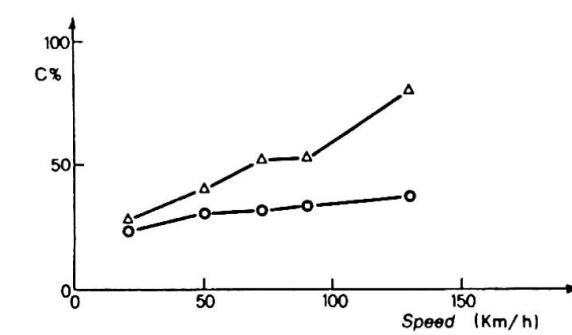
Fig. 10 -  $C_{overt}$  (○) and  $C_d$  (Δ) maximum values versus train speed
