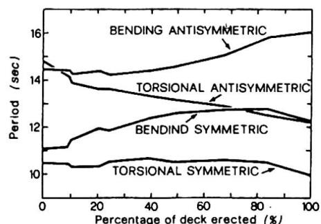
Fig. 12 - Natural frequencies evolution during the erection
