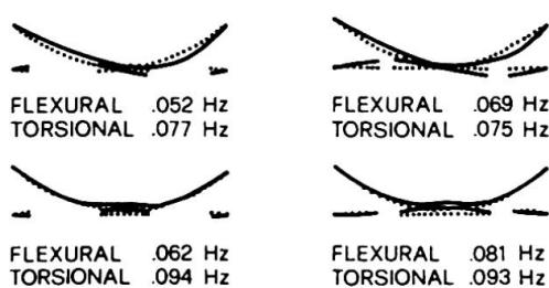
Fig. 11 - Mode shapes for deck erected at a) 30%, b) 80%
