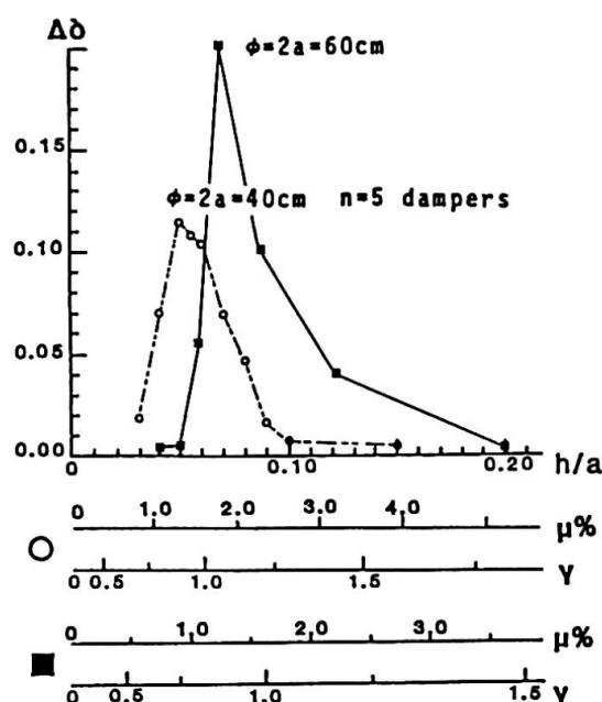
Fig. 5 Comparison of one large and five small TLDs ( $m_S = 440 \text{ kg}$ )
