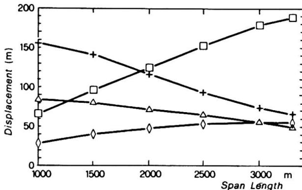
Fig. 1 - Maximum vertical displacements versus centre span length
