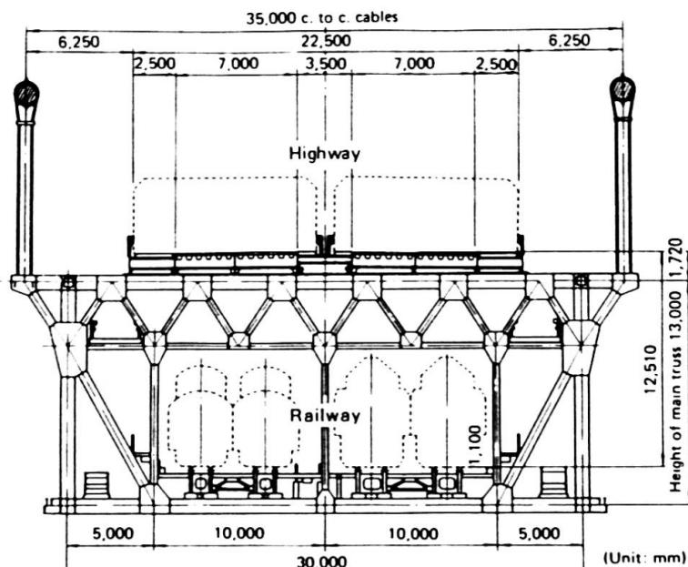
Fig. 2 Typical Cross Section of the Suspension Bridge
