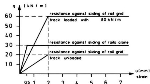
Fig. 1 Stress-strain diagram of ballast
