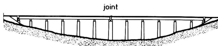
Fig. 6 Continuous girder bridge with one central joint
