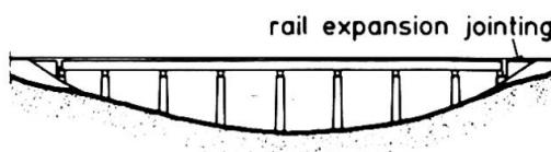
Fig. 5 Continuous girder bridge fixed at one end
