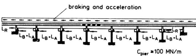
Fig. 2 Statical system and longitudinal forces of the elevated superstructure.
