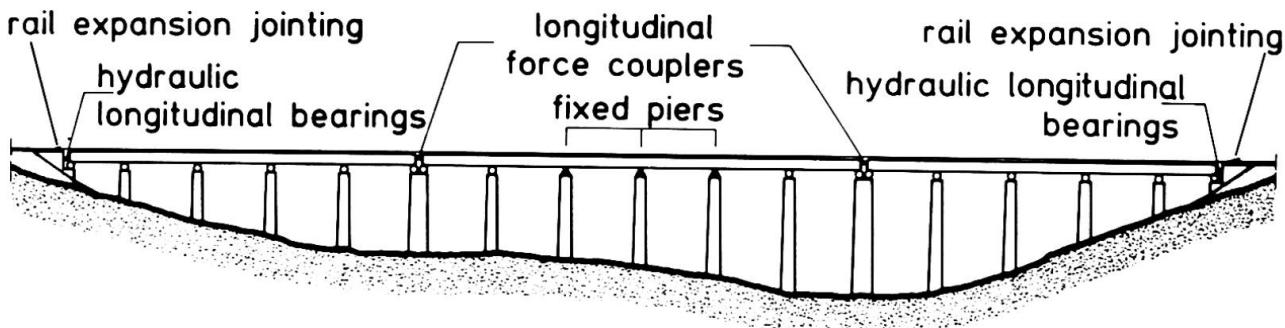
Fig. 7 Continuous girder bridge with hydraulic longitudinal bearings
