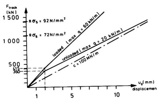
Fig. 3 Force-displacement characteristics of rail grids
