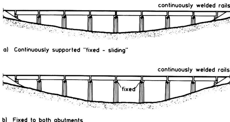
Fig. 4 Simple span valley bridges without special devices
