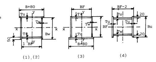
Fig.1 Notations of 2-span continous truss (unit:mm)
