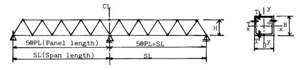
Fig.2 10-panel 2-Span continuous truss and notation
