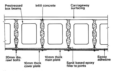
Fig. 2 Section on Deck
