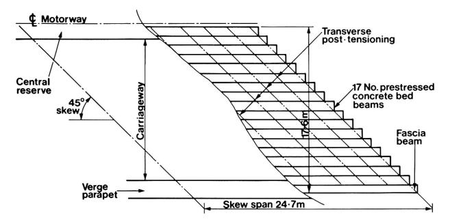
Fig. 1 Plan on Bridge Deck
