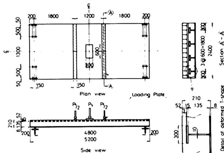
Fig. 6 Dimensions of specimen for fatigue test
