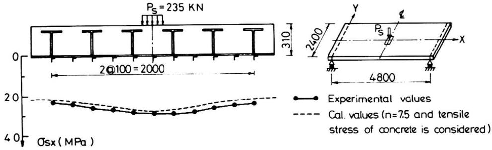
Fig. 7 Lateral distribution of tensile stress at mid-span section
