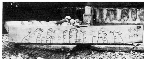
Photo.1 Failure mode of test beams
