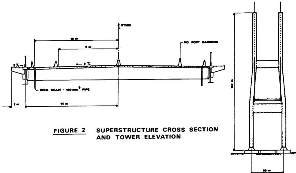
FIGURE 2 SUPERSTRUCTURE CROSS SECTION AND TOWER ELEVATION
