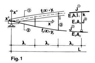
In some cases it is convenient to prestress the system to the necessary degree. However, due to deformations under dead and live load, a certain degree of self-prestressing is inherent to the system and is, in many cases, quite sufficient.
