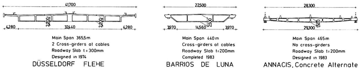
Fig. 2 Cross-sections of long-span cable-stayed concrete bridge beams
