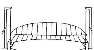
Now the air can be extracted from the concentrator housing thus created; with a partial vacuum between them the membrane surfaces will also withstand high wind loads.
