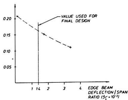
FIGURE 5 - HYPAR BUCKLING LOAD
