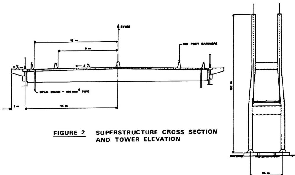
**FIGURE 2 SUPERSTRUCTURE CROSS SECTION AND TOWER ELEVATION**
