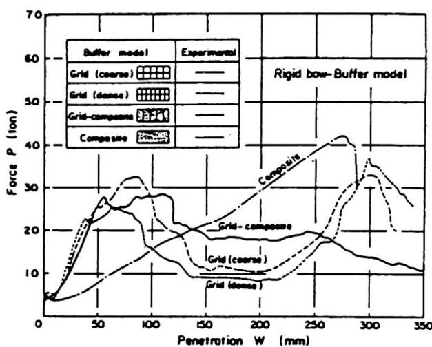
Fig. 3 Force-penetration curves of several kinds of buffer models
