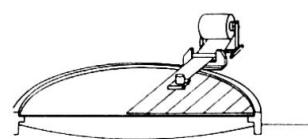
The membranes, which are 17 m in diameter, are made of individual sheet-metal strips welded together in the same plane with a welding device specially developed for thin sheet metal, which insures a gastight seam.
