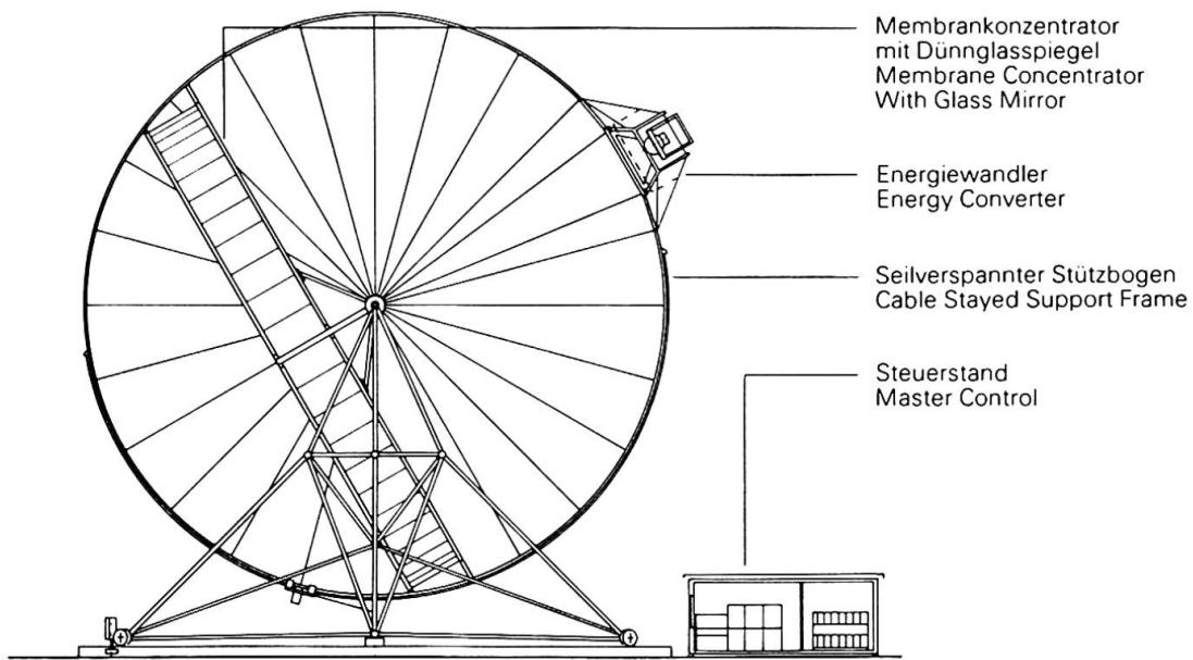
Fig. 6 A 50 kW solar power plant (see also Fig. 1).
