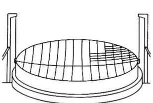
Finally, thin glass mirrors are bonded onto the front membrane.
