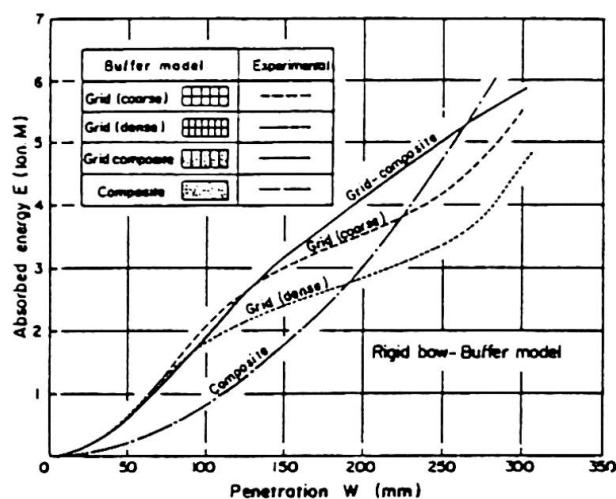
Fig. 4 Absorbed energy-penetration curves of several kinds of buffer models
