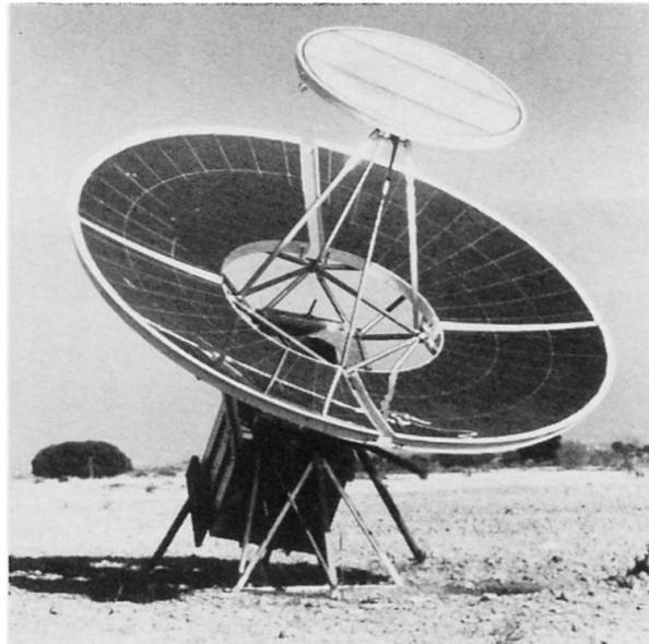
Fig. 5 A solar furnace for brick burning
