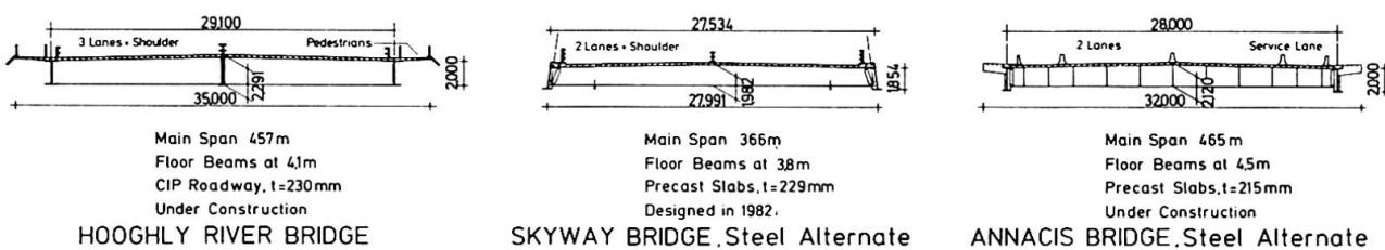
Fig. 3 Cross-sections of long-span cable-stayed composite bridge beams
