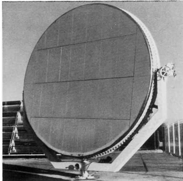
Fig. 4 Prototype of a membrane concentrator, 5 m diameter
