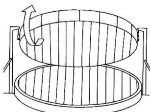
The front membrane is then deformed to a paraboloid by applying air pressure between the membrane and the ground and subsequently fixed to the ring.
