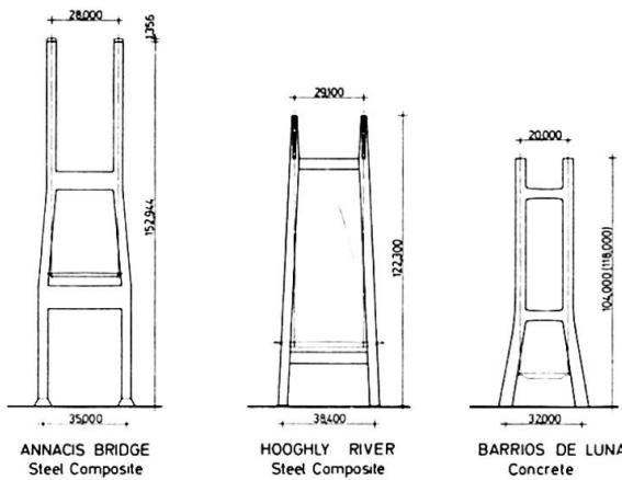
**Fig. 5** Tower shapes for recent long-span cable-stayed bridges
