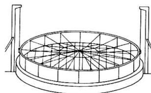
After fixing the rear membrane to the ring the concentrator is turned over.
