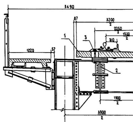
Fig.14. Deck elements connection by high strength bolts
