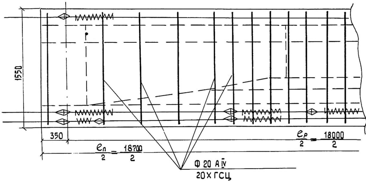
Fig.12. Reinforcement of superstructure
