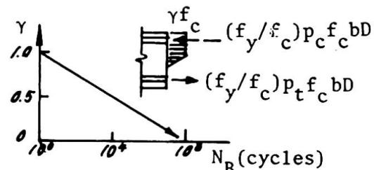
Fig. 7 Deterioration of concrete strength
