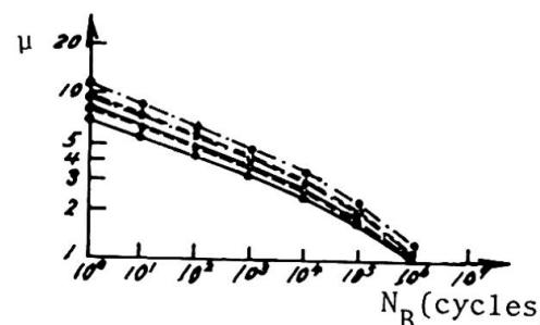
Fig. 9 Ductility factor-number of cycles to fracture
