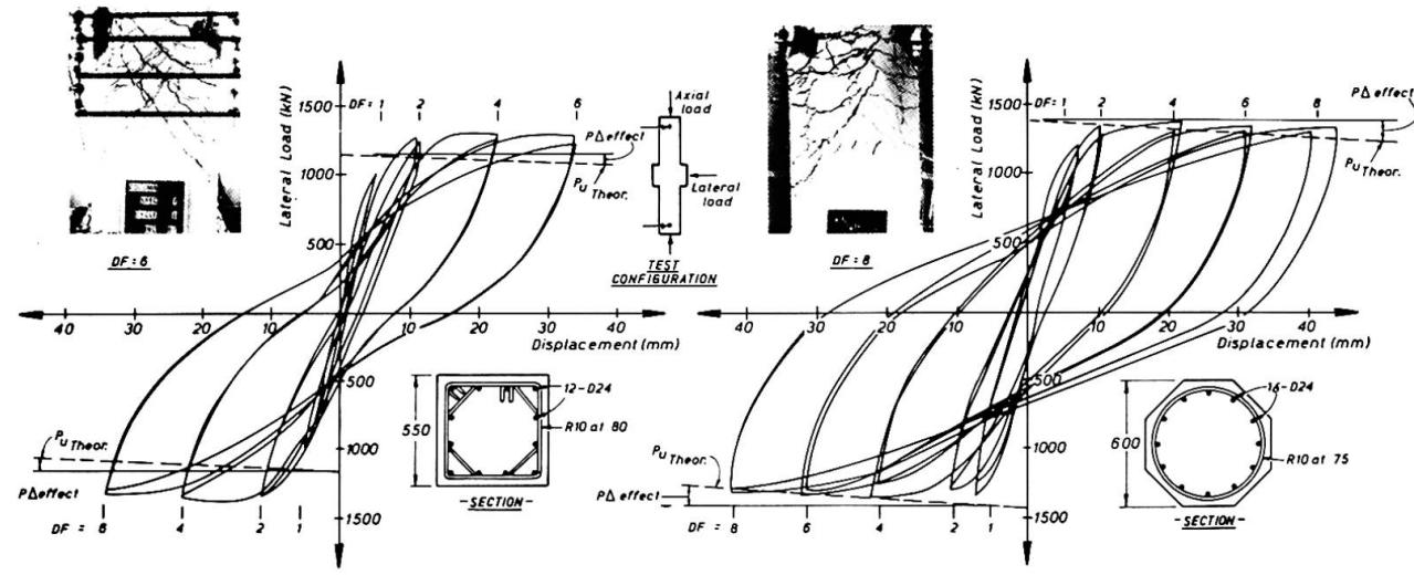
FIG. 5 - LOAD-DISPLACEMENT LOOPS FOR FULLY CONFINED COLUMNS
