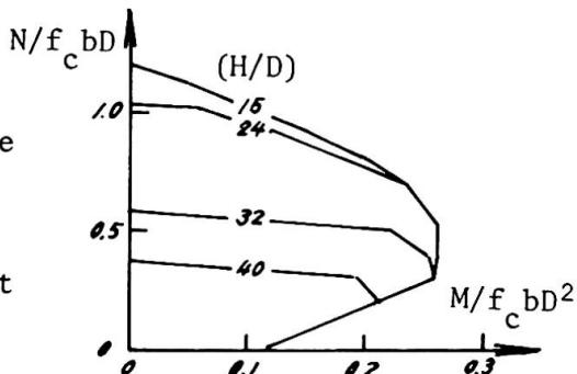
Fig. 10 Ultimate N-M-Interaction curve of long columns (LC)
