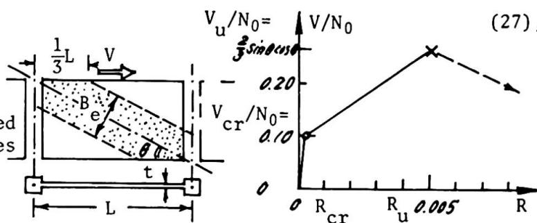
Fig.12 Shear walls (SW)
