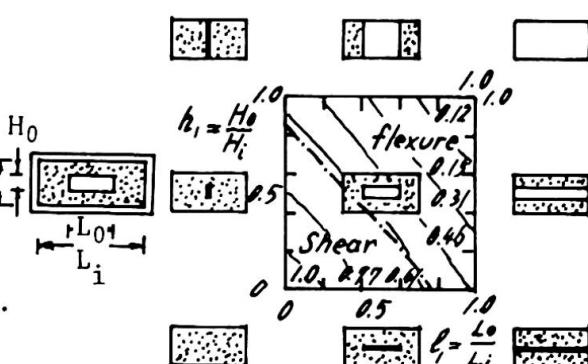
Fig.14 Ultimate resistances of shear walls with openings [6]
