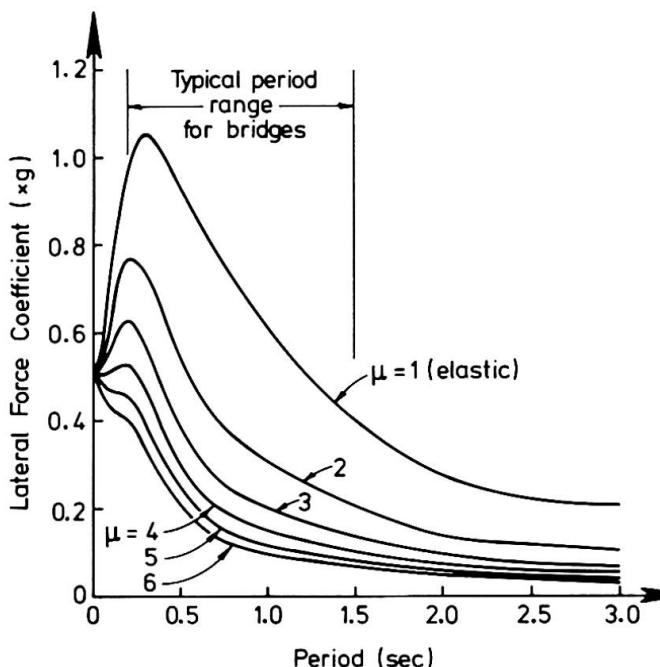
Fig. 1 INELASTIC DESIGN SPECTRA FOR
