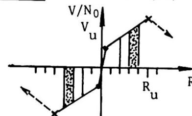
Fig.13 Hysteresis loop of shear wall
