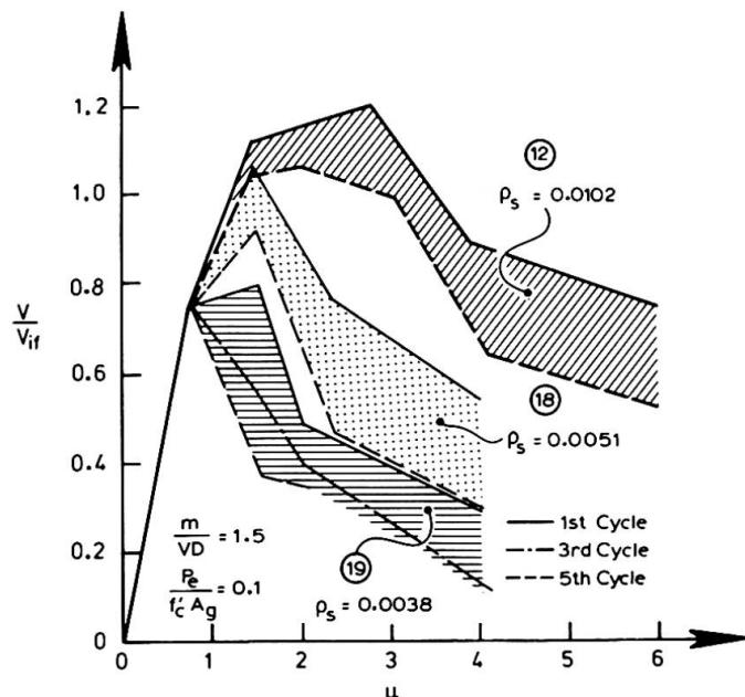
Fig. 7 DEGRADATION OF SHEAR STRENGTH WITH DUCTILITY
