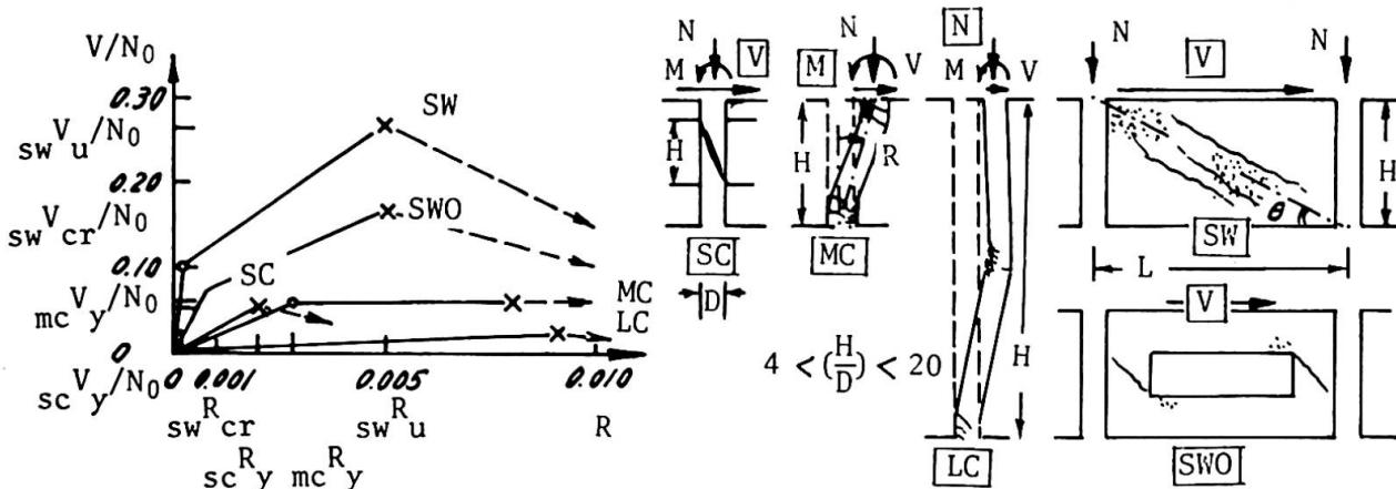
Fig.1 Resisting and deformation behaviours of aseismic elements
