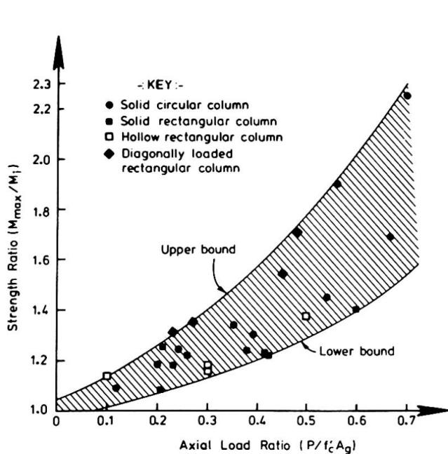
Fig. 6 FLEXURAL STRENGTH ENHANCEMENT OF CONFINED COLUMNS
