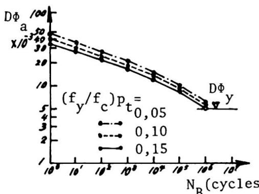
Fig. 8 Curvature amplitude-number of cycles to fracture
