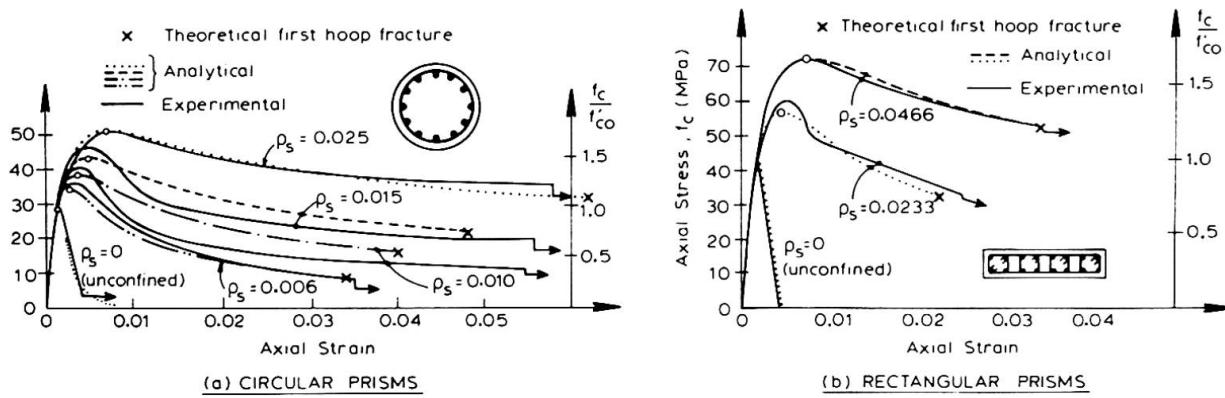
Fig. 4 AXIAL STRESS-STRAIN CURVES FOR CONFINED CONCRETE
