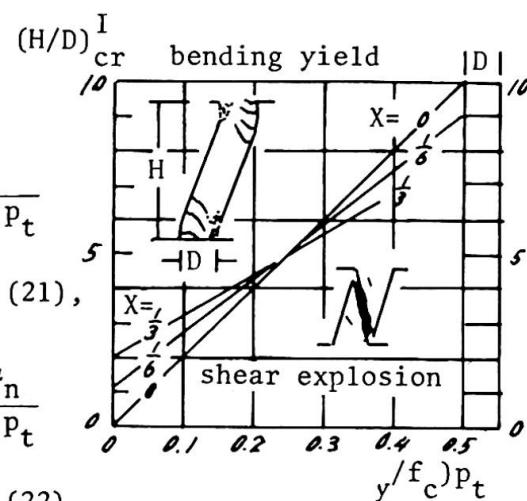
Fig. 11 Critical shear span ratio ( $H/D$ )<sub>cr</sub><sup>I</sup>
