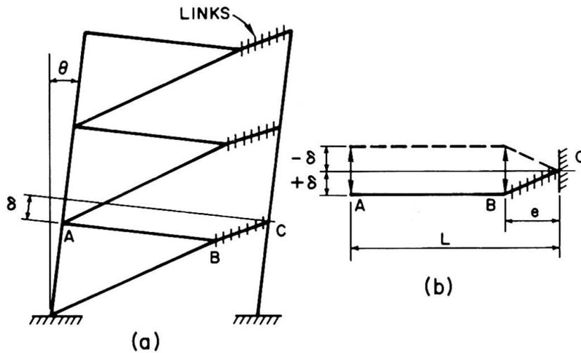
Fig. 10. (a) Collapse Mechanism of a Frame. (b) Schematic Diagram of Test Setup for Exterior Link.
