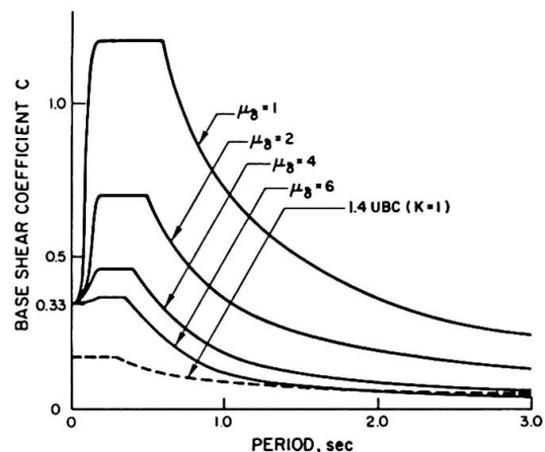
Fig. 1. Base Shear Coefficient Curves [20].
