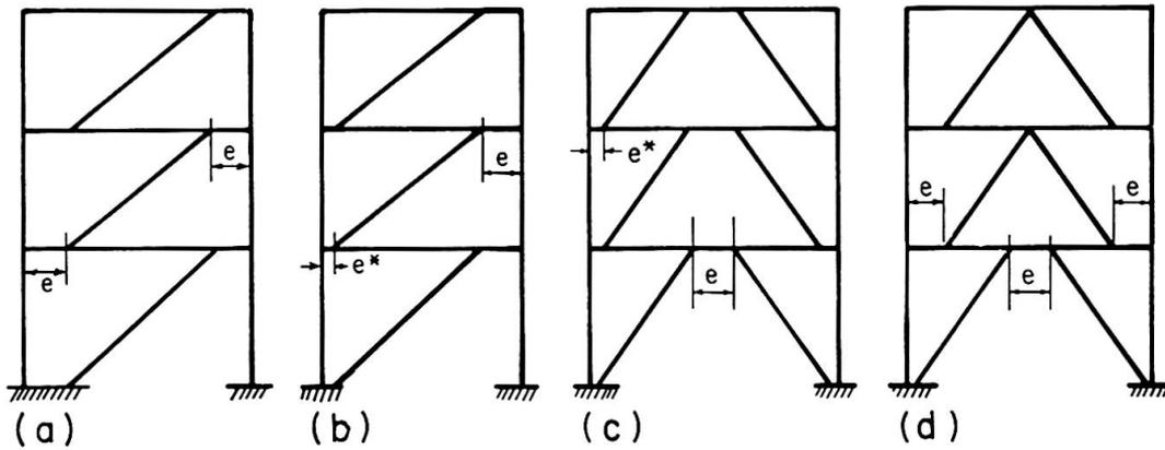
Fig. 8. Alternative Bracing Arrangements for Eccentrically Braced Frames [8].
