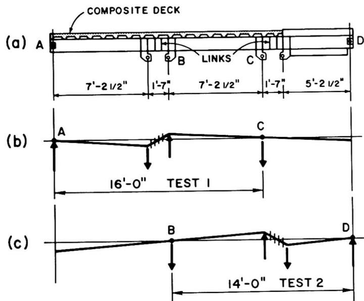
Fig. 11. (a) Composite Floor Beam with Links. (b) and (c) Schematic Diagrams of Test Setups for Interior and Exterior Links.
