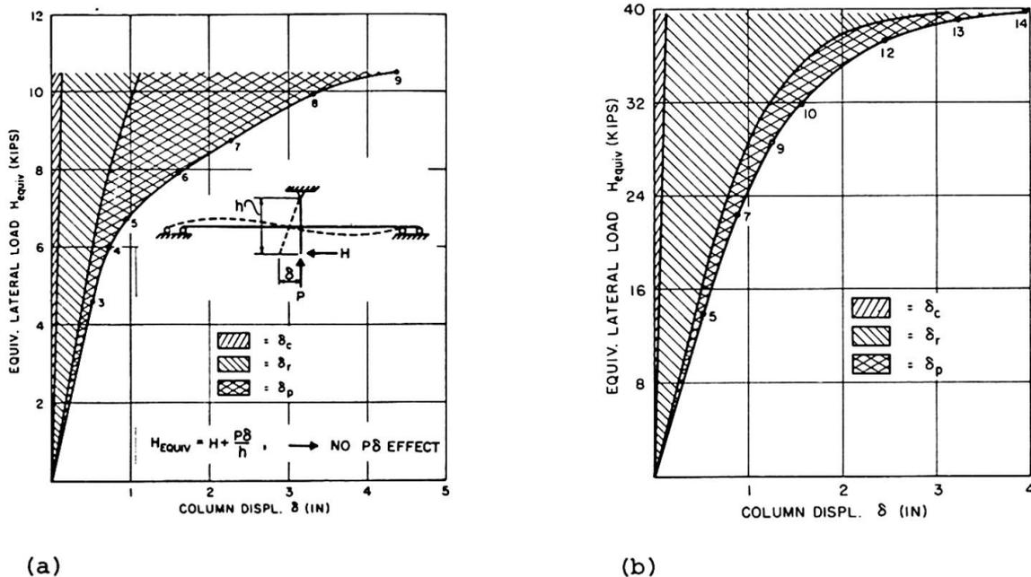
Fig. 5. Horizontal Displacement Components of Column with (a) Thin Web and (b) Thick Web [10].
