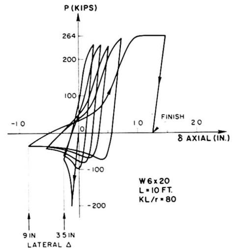
Fig. 6. Experimental Hysteretic Loops for Cyclically Loaded Strut [20].
