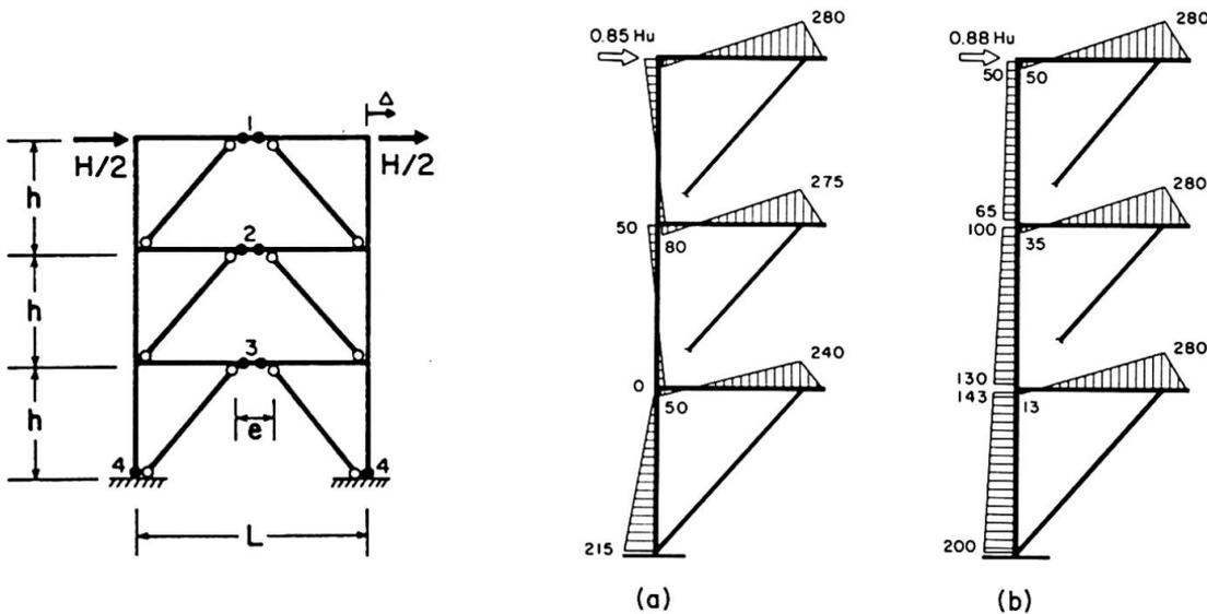
Fig. 3. Split K-Braced Frame. (a) Moments at First Yield. (b) Moments at Frame Ductility of 2 [8].
