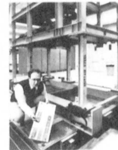
EXPERIMENTAL INVESTIGATION OF MODEL BUILDING ON EARTHQUAKE SIMULATOR
