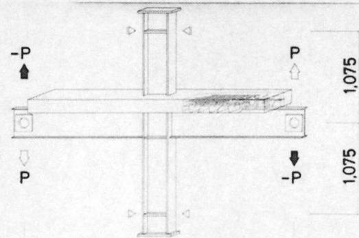
Fig. 1 Configuration of Specimens
