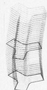
an example of analytical deformation magnified one hundred times
