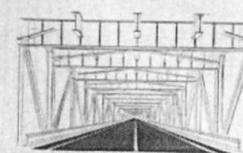
A THE VERTICAL MEMBERS ARE RIGIDLY CONNECTED TO A BOX GIRDER.
