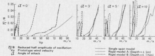
The original section was suspected to have unstable aerodynamic behavior, so, wind tunnel tests were conducted to reveal that the original section had vortex-induced oscillation at the wind speed of 15 to 20 m/s and galloping which should not occur below the speed of 92 m/s (10minutes average), the dynamic design wind speed.
