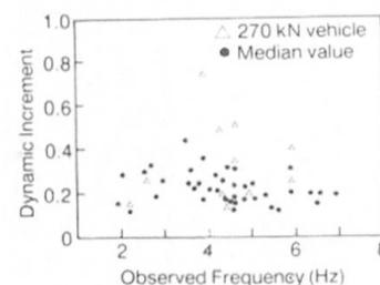
**Dynamic load allowance** is a fraction of highway live load to cater for dynamic effects of vehicle & bridge, and riding surface irregularity.
