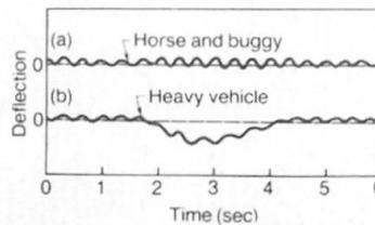
Typical field data for dynamic amplification indicate considerable scatter due to variation in vehicle type and pavement roughness. Mean amplification tends to increase with speed and to increase with bridge frequency in the range 2 to 5 Hz - typical of the bounce frequency of modern heavy vehicles (below). The results lend themselves to a statistical treatment.
