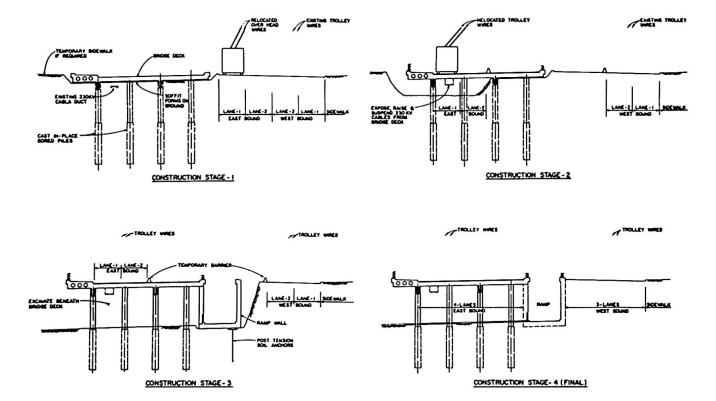
FIGURE 3/OAKRIDGE CENTRE: 41ST AVENUE BRIDGE-CONSTRUCTION STAGES
