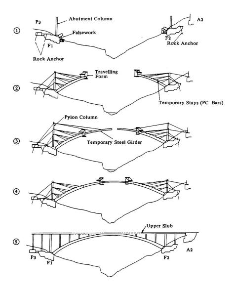
Fig. 2, Construction Process
