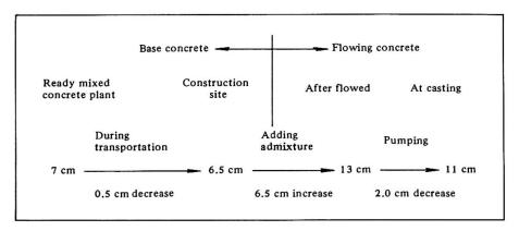
Fig. 4. Slump Change of Concrete
