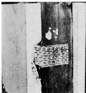
Fig. 16.5 Final failure by cracking of concrete edge for no. 5
