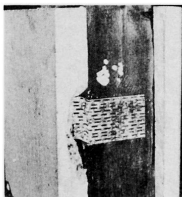
Fig. 16.5 Final failure by cracking of concrete edge for no. 5
