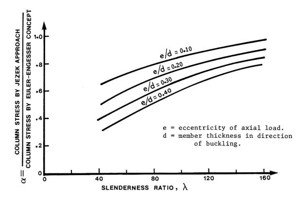
Fig. 2 Effect of Loading Eccentricity on Column Strength
