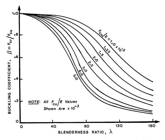
Fig. 4 Buckling Coefficient versus Slenderness Ratio Curves
