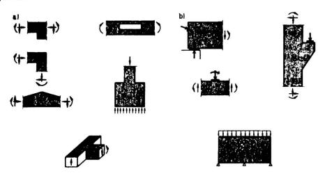
Fig. 1 (a) Geometrical discontinuities, (b) statical and/or geometrical discontinuities
