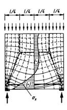
Fig. 6 The strut model approximating the stress trajectories
