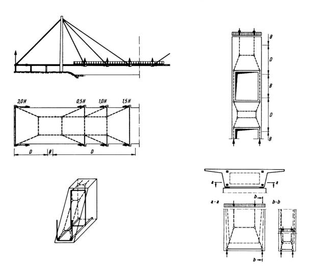
Fig. 7 One single type of a D-model appears in 4 different structures
