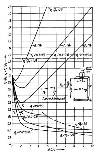
Fig 11 Diagram for evaluating the critical load of plane compression bars (\$\beta\_n\$ = prism strength)
