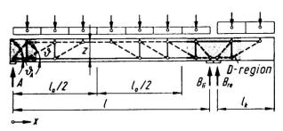
Fig. 2 Truss model of a beam with cantilever
