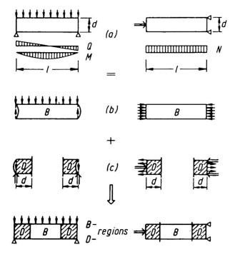
Fig. 4 Splitting of structure into B- and D-regions
