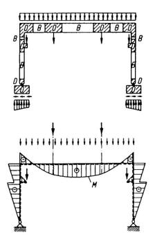
Fig. 5 Frame structure with B- and D-regions
