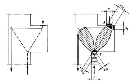
Fig. 13 Compression bars (fields) of a corbel
