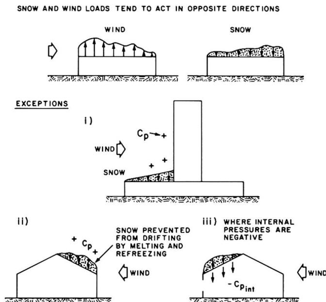
Fig. 5 Combined Snow and Wind Loads on Roofs
