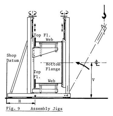
Two rolling frames (Fig. 10) were located at approximately the one-fifth point from each end and secured around the box after passage of the automatic welding machines. The boxes were then rotated through 180° for completion of the web-to-flange welds and rotated to intermediate positions for optimum welding of internal stiffeners, gussets, cross-bracing, etc.
