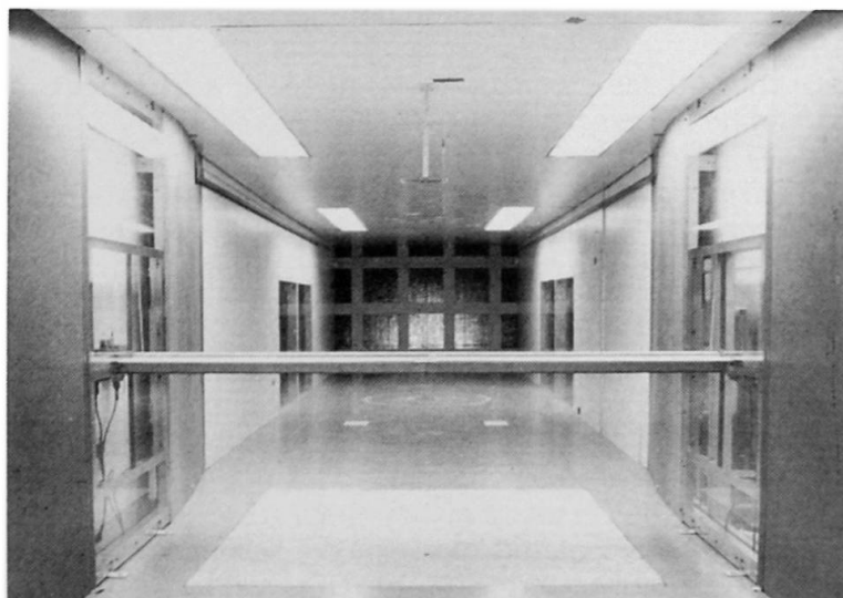
Fig. 5 Section Model in Wind Tunnel
