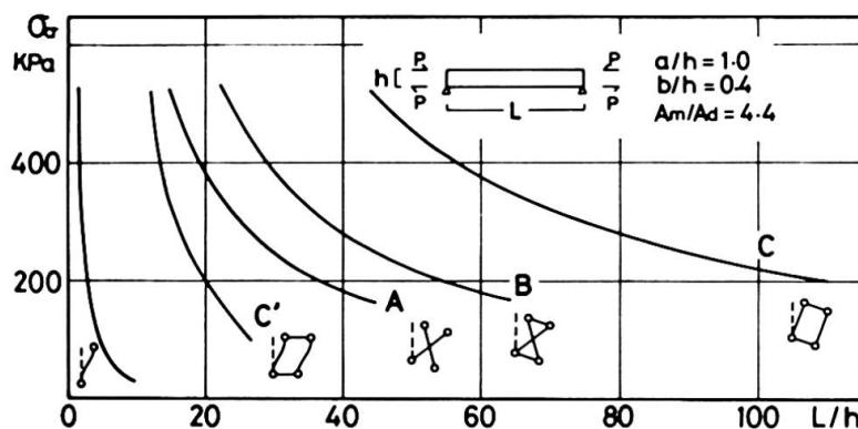
Fig. 2 Lateral buckling strength of lattice beams
