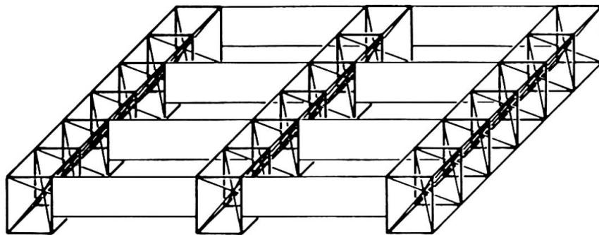
Fig. 1 Wide-span structures using beam-like lattice trusses
