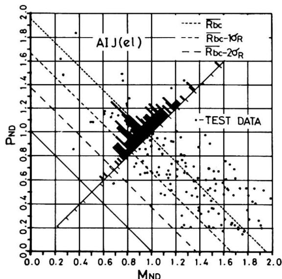
Fig. 11 Test data based on AIJ(e1) spec.
