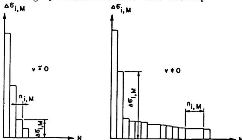
Fig. 6 Multi-stage spectrum
