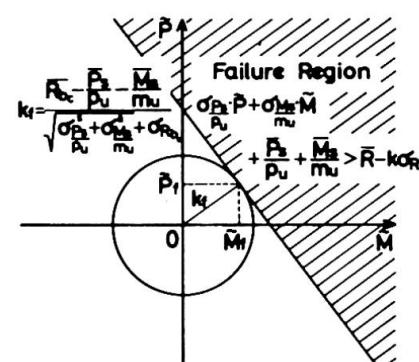
Fig.1 Failure criterion Fig.2 Equivalent resistance Fig.3 Failure criterion
