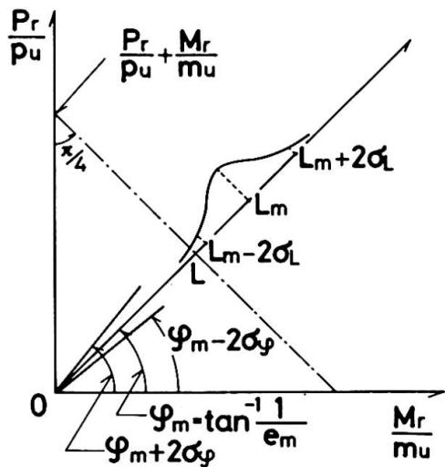
Fig. 8 Evaluate method of resistance of beam-column
