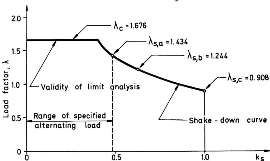
Fig. 5 Range of limit analysis and shake-down validity
