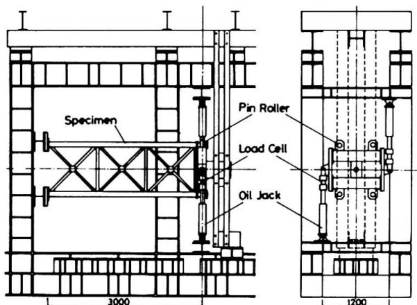
Fig. 4 Set-up of model experiment under torsion
