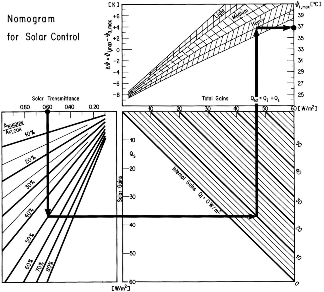
Fig. 7: Nomogram for solar control (Swiss climatic conditions)
