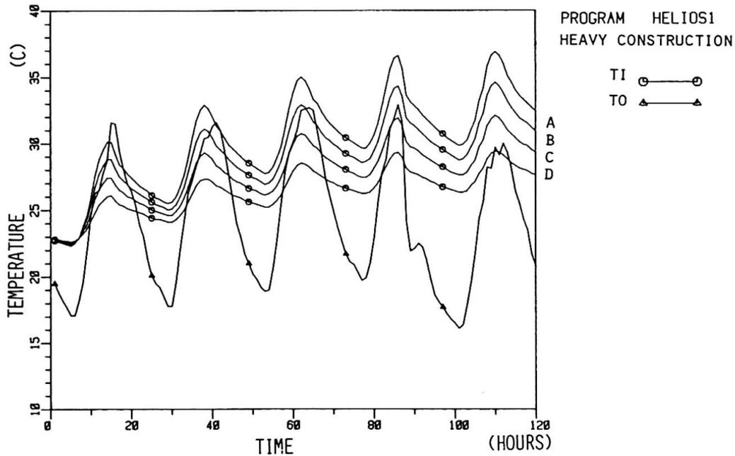
Fig. 4: Calculated indoor air temperatures of a heavy building construction for different ratios of window to floor area  $A_w/A_f$ : A=50%, B=40%, C=30%, D=20%.
