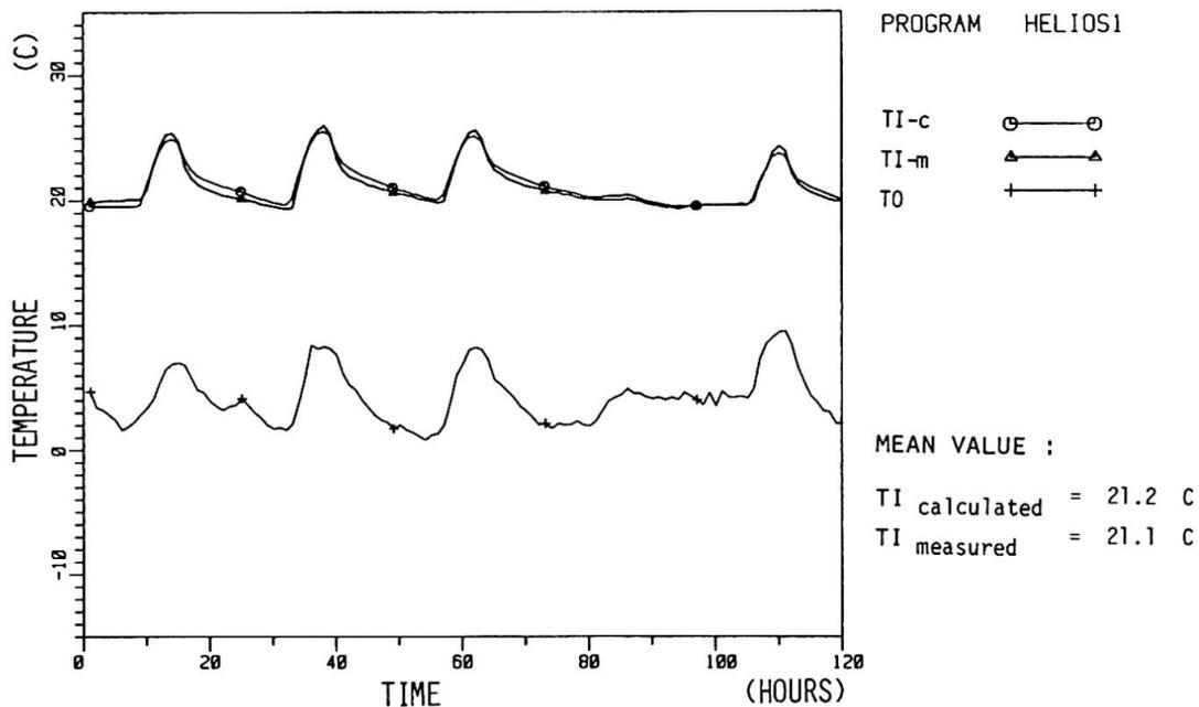
Fig. 3: Comparison of measured and calculated indoor air temperature for a south oriented room.
