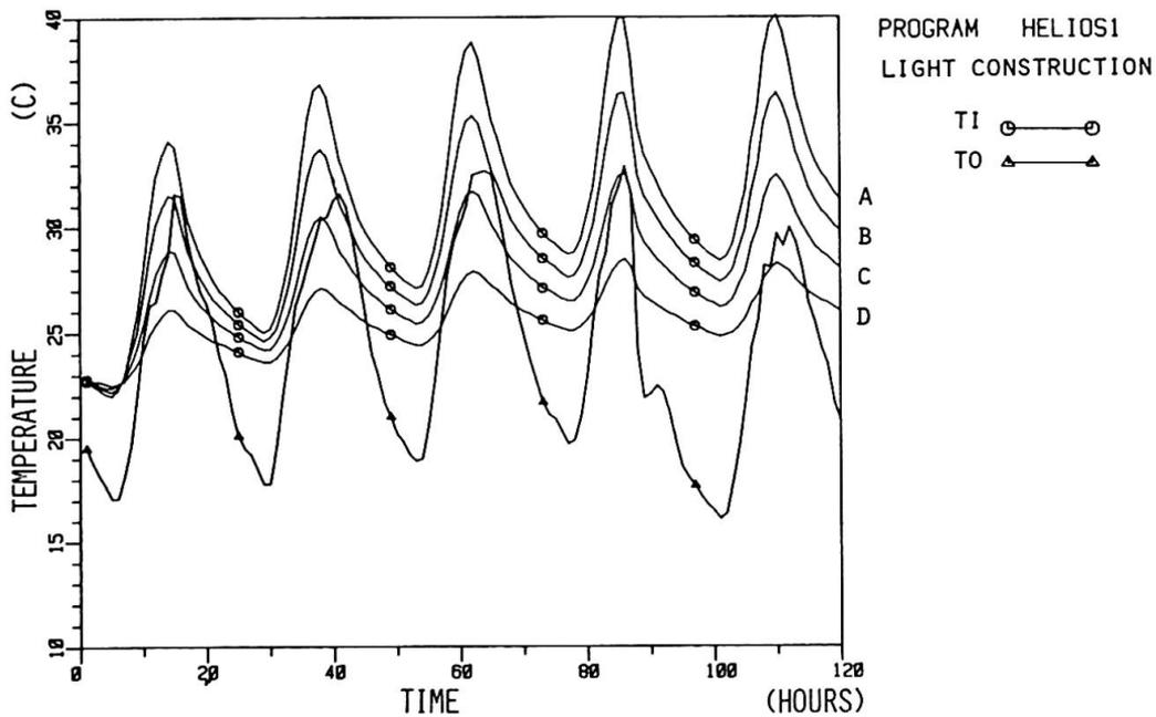
Fig. 5: Calculated indoor air temperatures of a light building construction for different ratios of window to floor area  $A_w/A_f$ : A=40%, B=30%, C=20%, D=10%.
