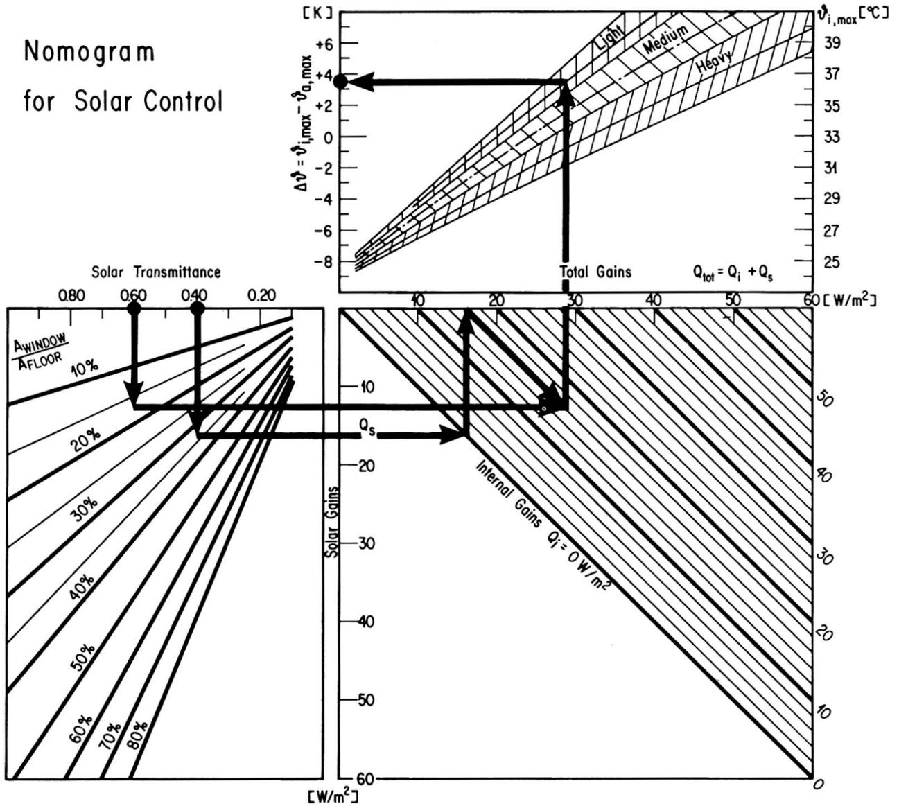
Fig. 8: Nomogram for solar control (Swiss climatic conditions)
