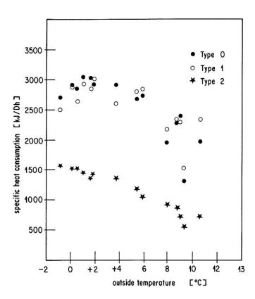
In the type 2 building with the microprocessor control system, the values are increasing monotonously with lower outside temperatures and with a much smaller scatter, showing that the temperature control is really done by the control system in an energy efficient way.
