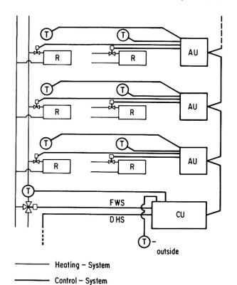
Fig. 2: Schematic view of the control system
