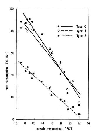
Fig. 4: Energy signatures of the three test buildings
