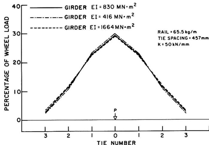
Fig.3. Effect of girder stiffness on load distribution
