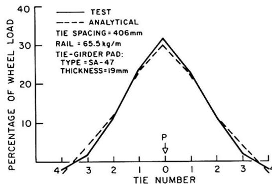
Fig.8. Comparison of test data with analytical prediction
