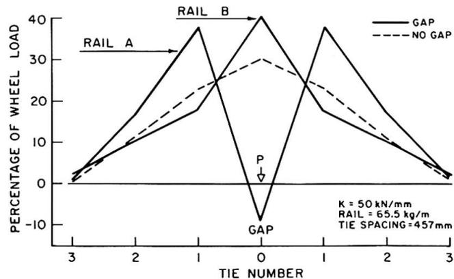
Fig.6. Effect on load distribution of a gap at the central tie
