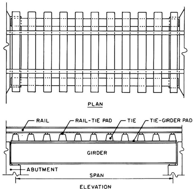
Fig.1. Open deck railway bridge with concrete ties
