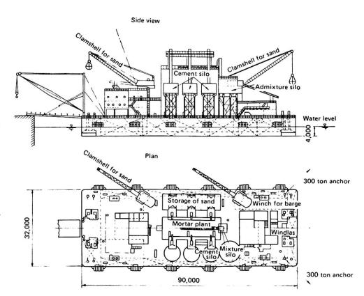
capacity of Fig. 6 General View of the Mortar Plant Vessel  $6,000 \text{ } \ell/\text{min}$ . has been built in 1978 and is now ready to be used.
