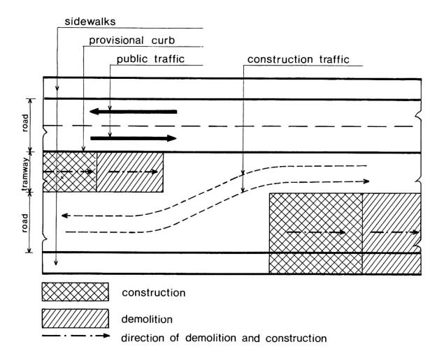
Fig. 3. The construction phases.
