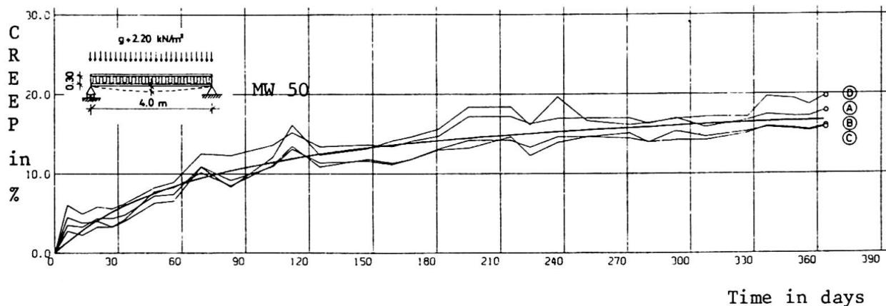
In the short term load tests with centrally and eccentrically loaded wall-components these were 2.4 m high and 1.2 m wide. The components had no web-plates. In the tests with 20 cm thick wall-components the following results were found:
