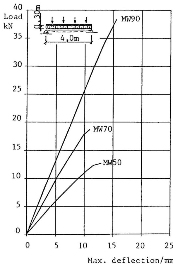
Failure occurred as shear failure between skin and core close to the supports.
