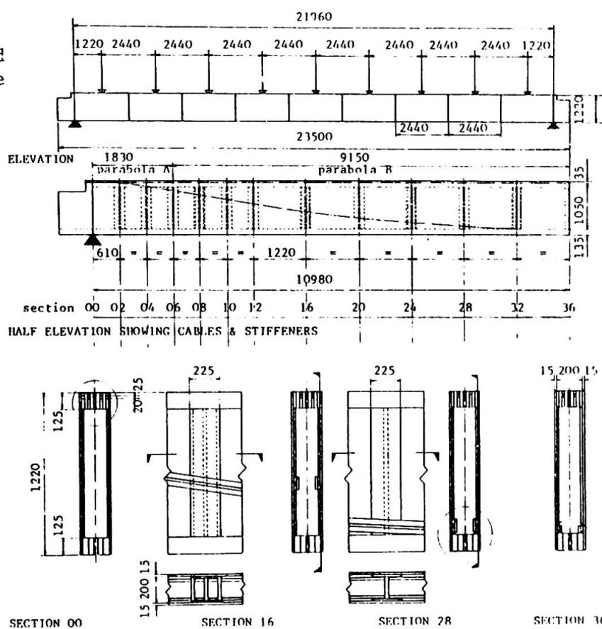
Fig. 2 General arrangement of beam and stressing system
