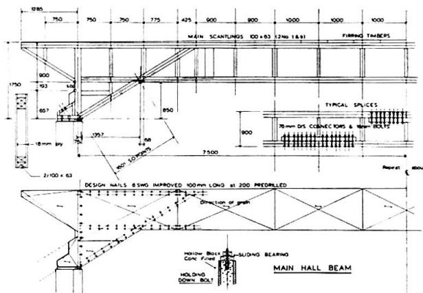
Fig.4: Drawing of 15m span main hall beam.
