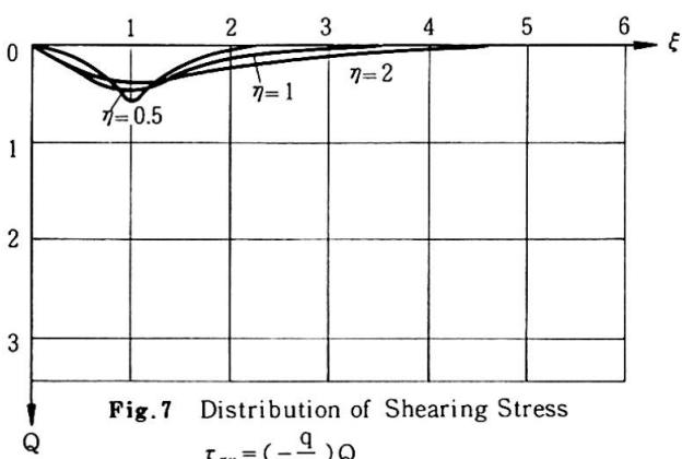
**Fig. 7** Distribution of Shearing Stress
