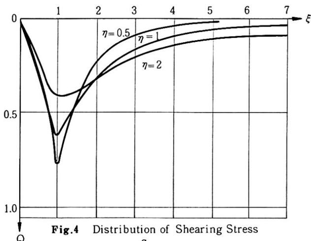
**Fig. 4** Distribution of Shearing Stress
