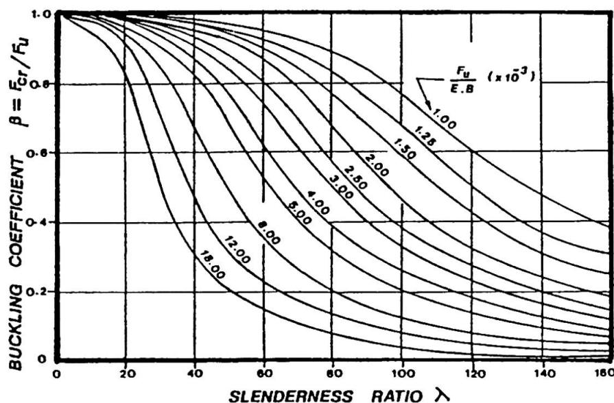
Fig. 3 Buckling Coefficient Versus Slenderness Ratio Curves
