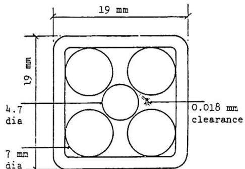
Fig. 3 Compressed cable form
