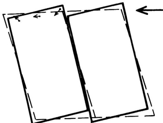
Fig. 1 Wall element with two board panels loaded in shear. Schematic illustration of deformations. The small arrows show the deformation of the nails from board to timber frame.
