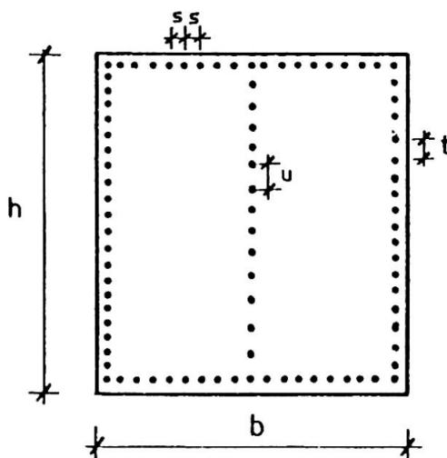
**Fig.4** Definition of non-dimensional parameters  $n$ ,  $m$ , and  $p$  for fastener spacing for a wall with three vertical studs.
