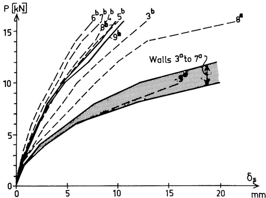
Fig. 3 Load versus measured horizontal displacement at upper unloaded corner (point 5).
