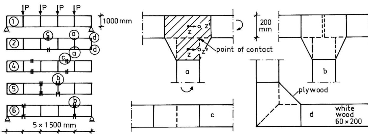
Fig. 1 Places member joints: 11, and plywood gussets.
