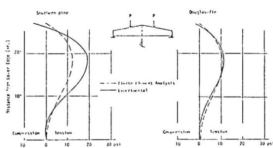
Fig. 6 Radial Stress for 27" Beams
