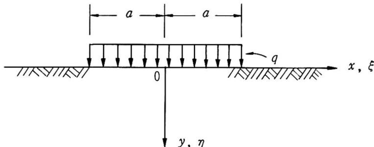
Fig. 1 Partial Uniform Load on an Half- infinite Orthotropic Material
