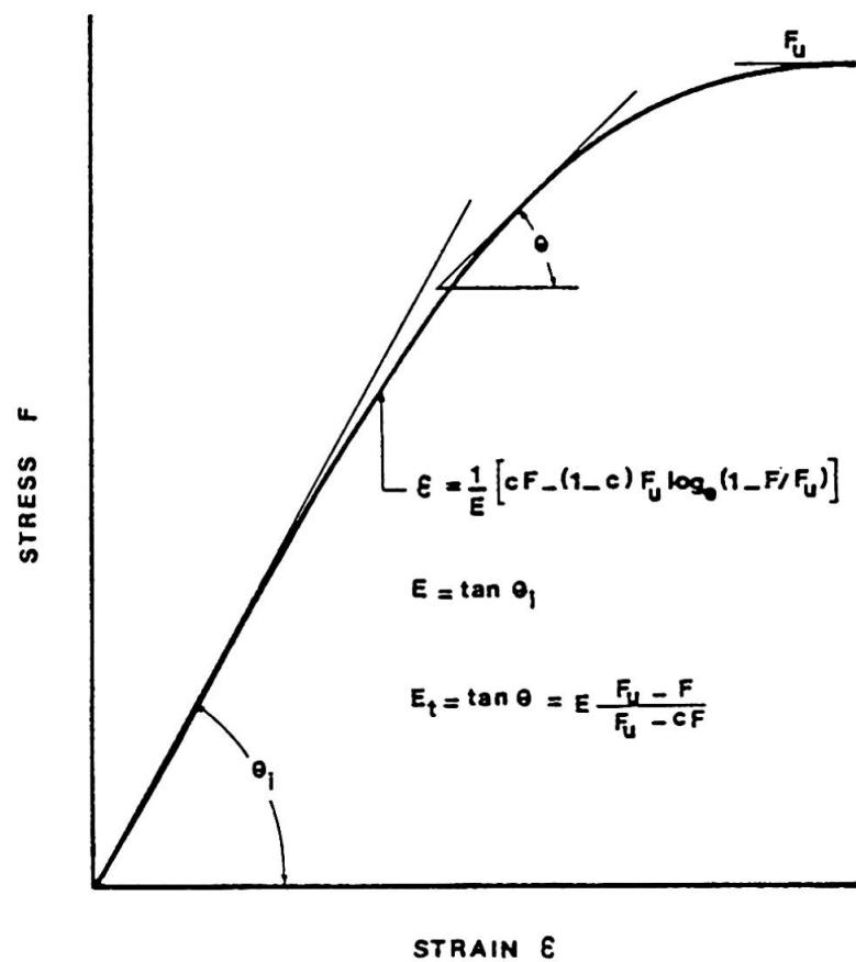
Fig. 1 Stress-Strain Curve
