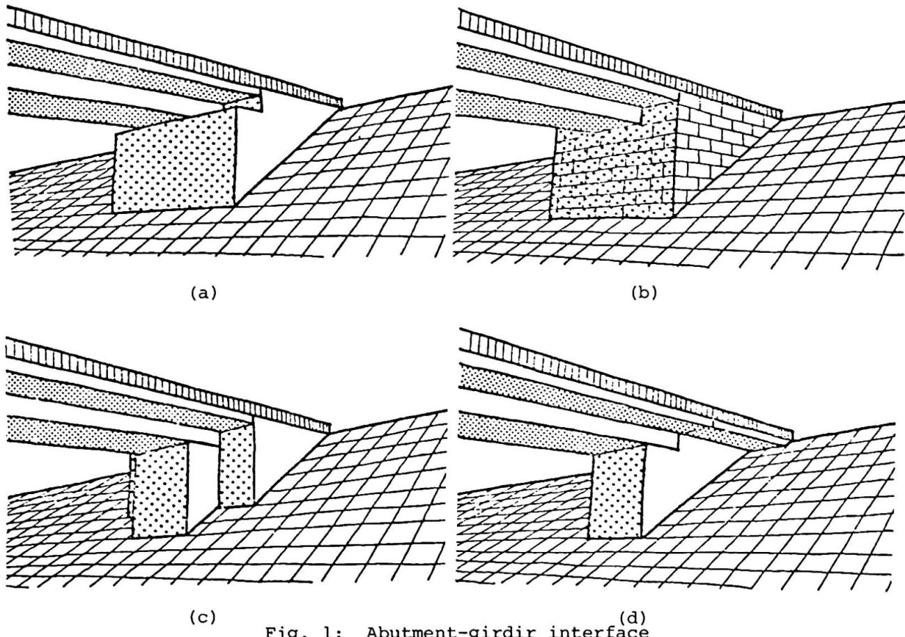
Fig. 1: Abutment-girdir interface
