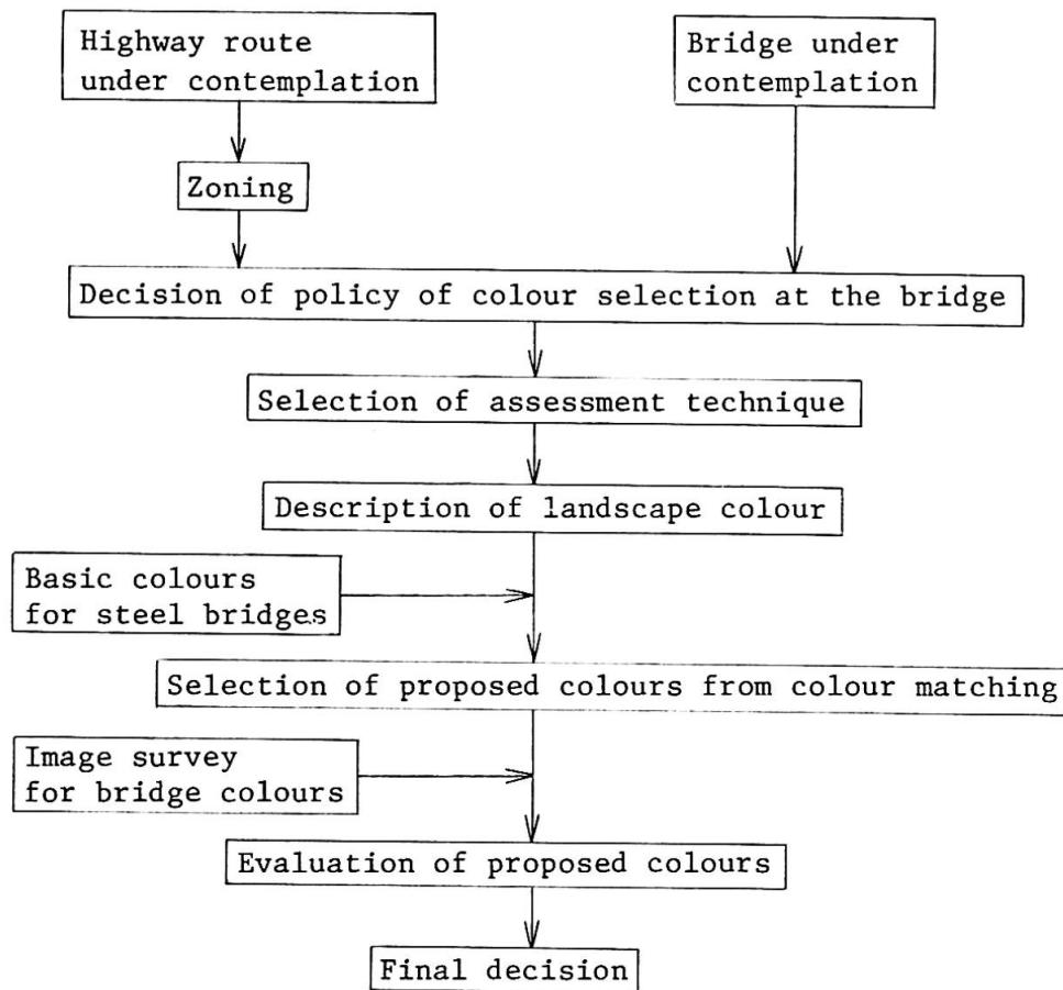
Fig. 1 Flow Chart of Colour Selection Procedure
