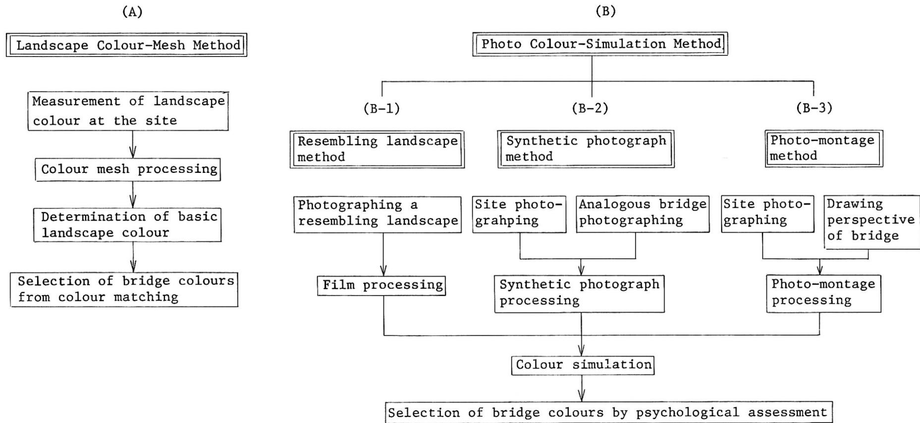
Fig. 2 Colour Selection Methods for Steel Bridges
