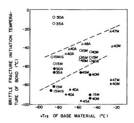
FIG. I RELATION BETWEEN THE BRITTLE FRACTURE INITATION TEMPERATURE (n=2.0) AND vTrs OF BASE MATERIAL
