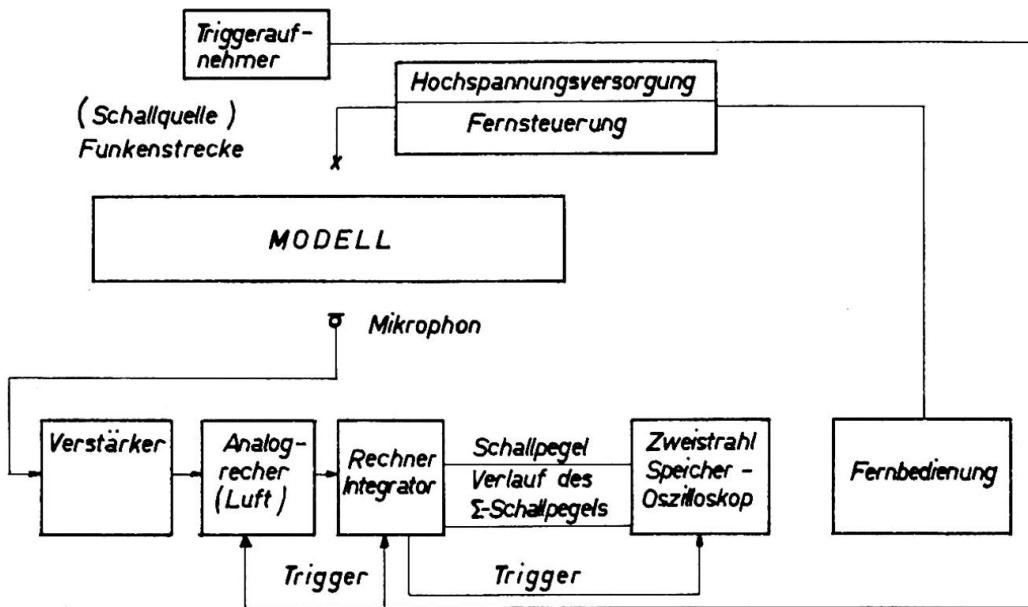
Fig. 3: Block diagram of measuring equipment for acoustic models
