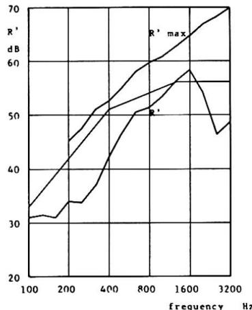
b) sound reduction measured in laboratory
