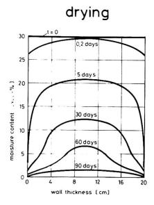
Fig. 5 Distribution of moisture concentrations on a wall of cellular concrete at different instants, according to [6].
