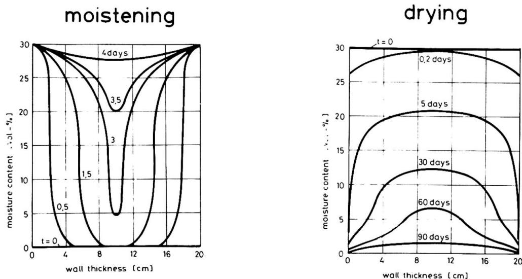
Fig. 5 Distribution of moisture concentrations on a wall of cellular concrete at different instants, according to [6].
