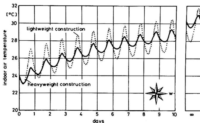
Thermal cyclic behaviour of a west-orientated room of light and heavy construction, according to [3].
