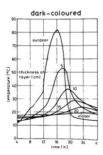
Fig. 3 Thermal stress of outer wall with light and dark colour, according to [5].
