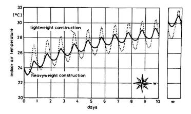
Thermal cyclic behaviour of a west-orientated room of light and heavy construction, according to [3]. Basic data 40 % window surface clear insulation glazing with outer blind change of air 0,5 h<sup>-1</sup>
