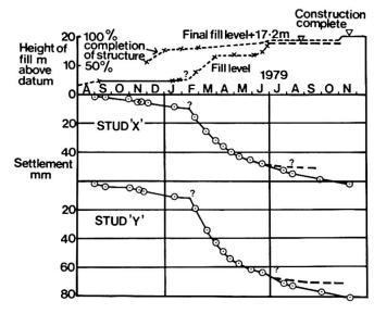
Figure 6 Loading and settlement with time.
