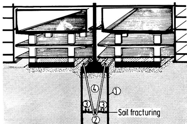
Fig. 5 Cement injection - soil fracturing method
