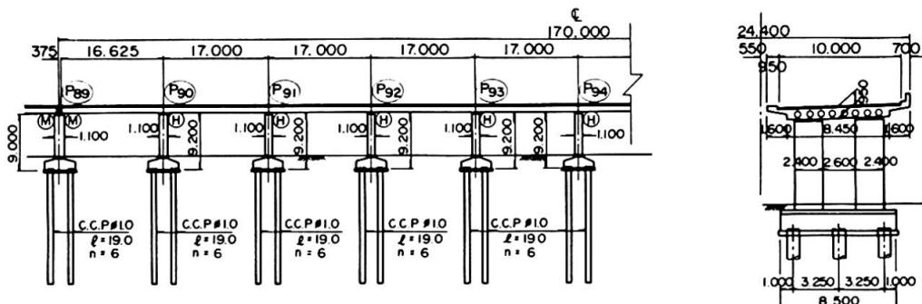
Fig. 4 General View of 10 Span Continuous Bridge
