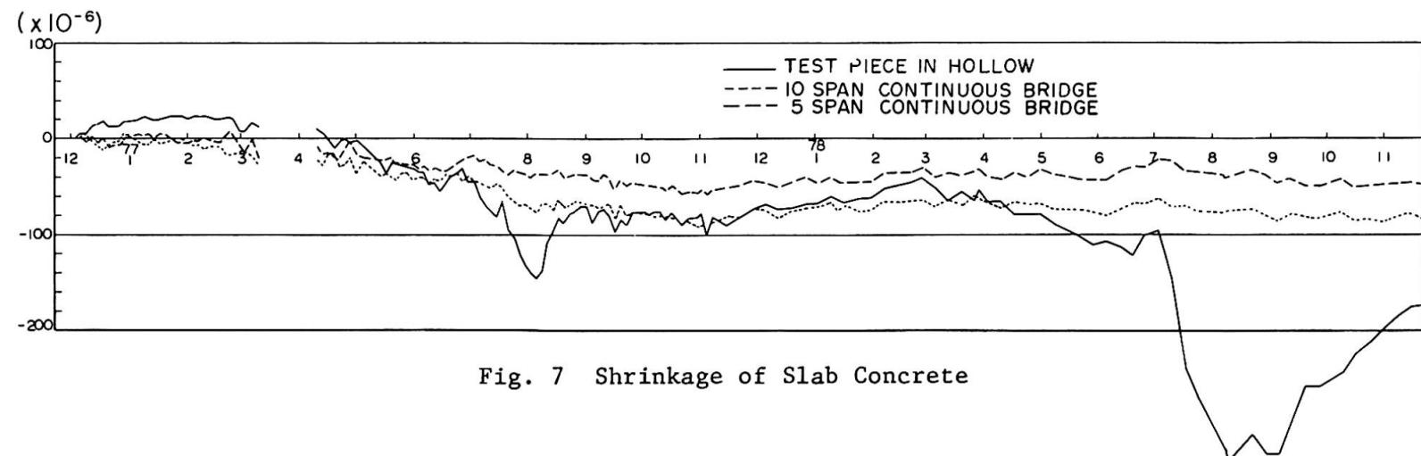
Fig. 7 Shrinkage of Slab Concrete
