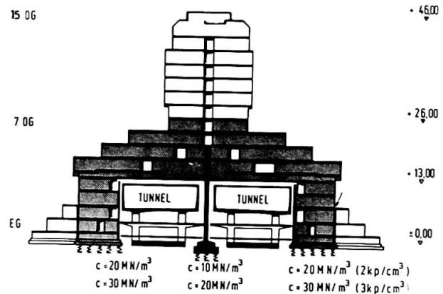
Fig. 2 Cross-section, foundation-moduli
