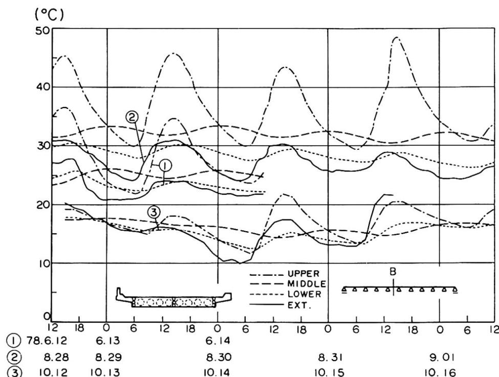
Fig. 10 Temperature Variation of Slab Concrete a Day
