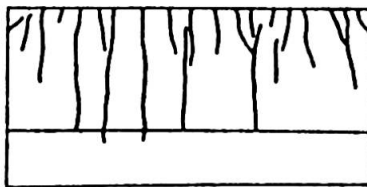
Fig. 3(a) Crack pattern development of A-5 (skin reinforcement = eight #3 bars)
